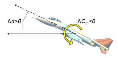
For stability, we need a *negative* change of the pitching moment if there is a *positive* change of the angle of attack (and vice versa), so:
