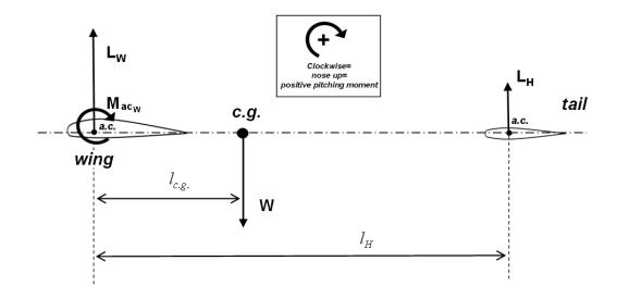
In this figure  $L_H$  is drawn upward. In reality it could just as well be pointed downwards, but the sign convention is that the lift is positive upward, and therefore we draw it like this.
