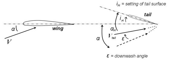
The wing has pushed air down and decreased the angle of attack with  $\varepsilon$ , the downwash angle.
