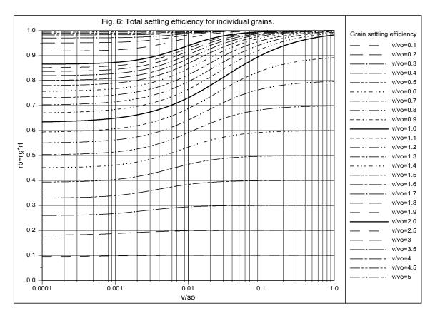
It is however of interest how the removal ratio (settling efficiency) of a grain can be split up in a part determined by laminar flow in the basin according to equation (12) and a part
