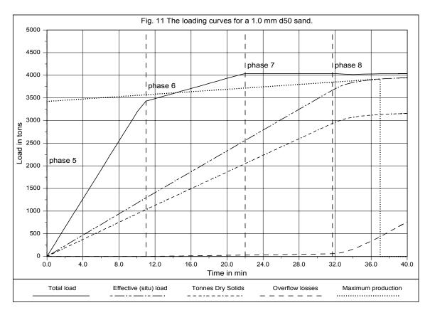
With these equations the hopper cycle for the net weight and the TDS can be derived, this is shown in the figures 8 to 11. The hopper dredge is optimally loaded, when the effective load (weight) or the TDS divided by the total cycle time  $dW_s/dt$  reaches its maximum. This is shown in figures 8 to 11 and is the reason for the starting point of the loading cycle in figure 8.
