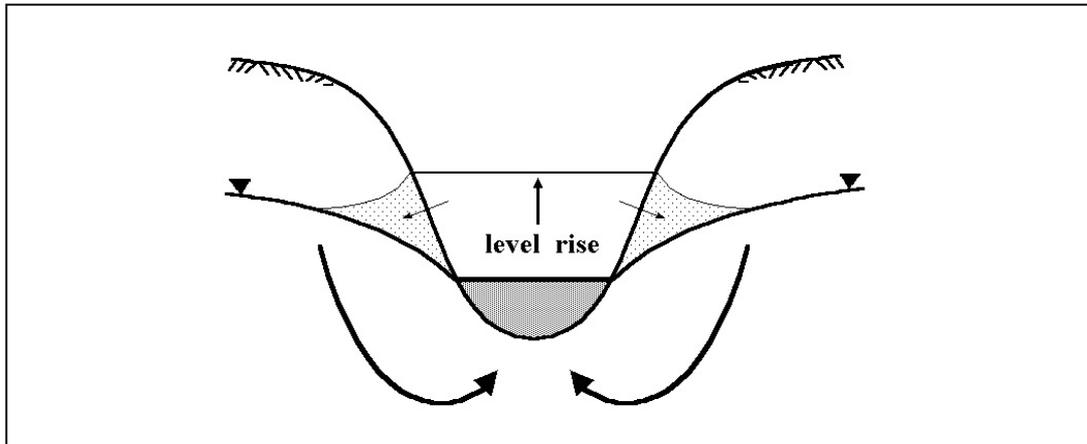
Figure 2.8: Temporary change of river, from effluent to influent due to a sudden rise of the water level
