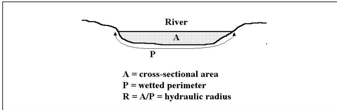
Figure 2.4: Cross-section of a river
