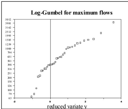
Figure 2.14: Log-Gumbel distribution for maximum flows in the Incomati river at Ressano Garcia
