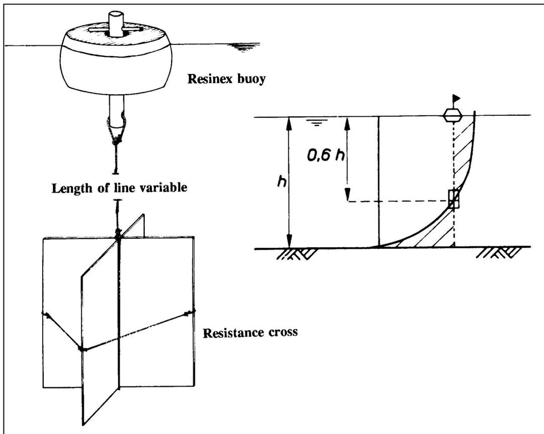
Figure 2.2: Float with resistance body, and location of the resistance body in the vertical
