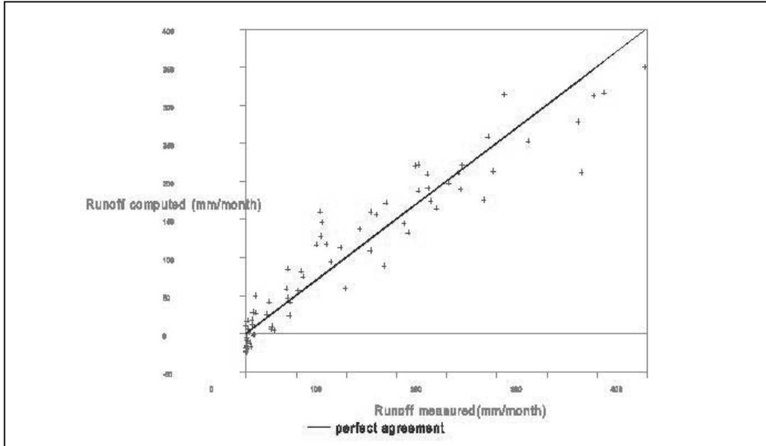
Figure 2.25: Measured versus computed runoff in the Cunapo catchment ( $D = 120$ )
