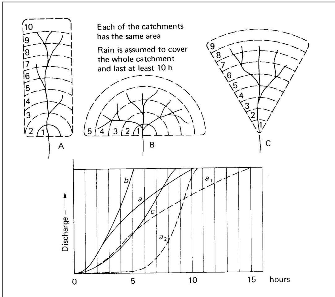
Figure 2.10: The effect of shape on catchment runoff (after Wilson, 1983)
