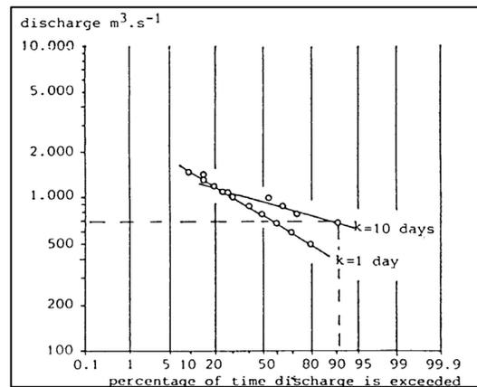
Figure 2.12: Flow duration curve on log-probability paper for flow durations of  $k = 1$  and  $k = 10$  days
