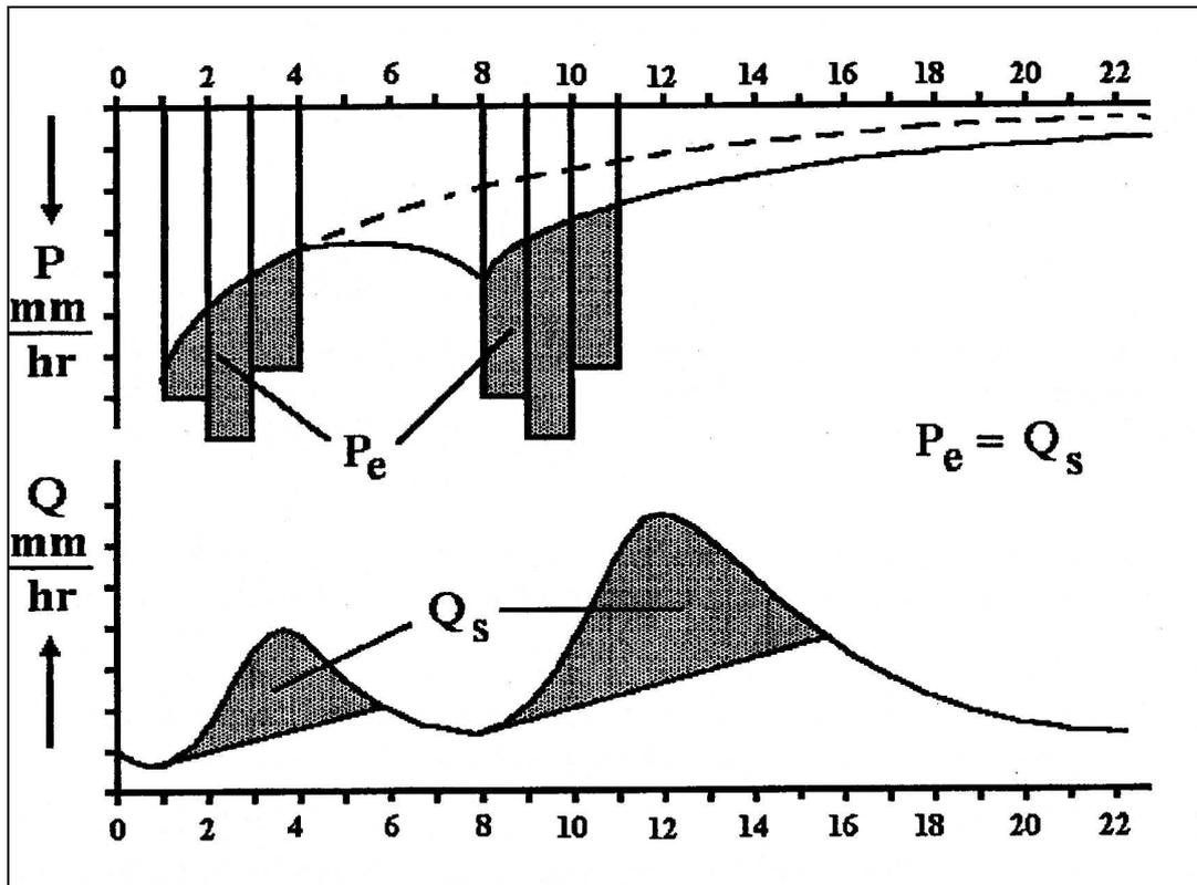
Figure 2.19: The effect of infiltration losses on the effective precipitation and direct runoff
