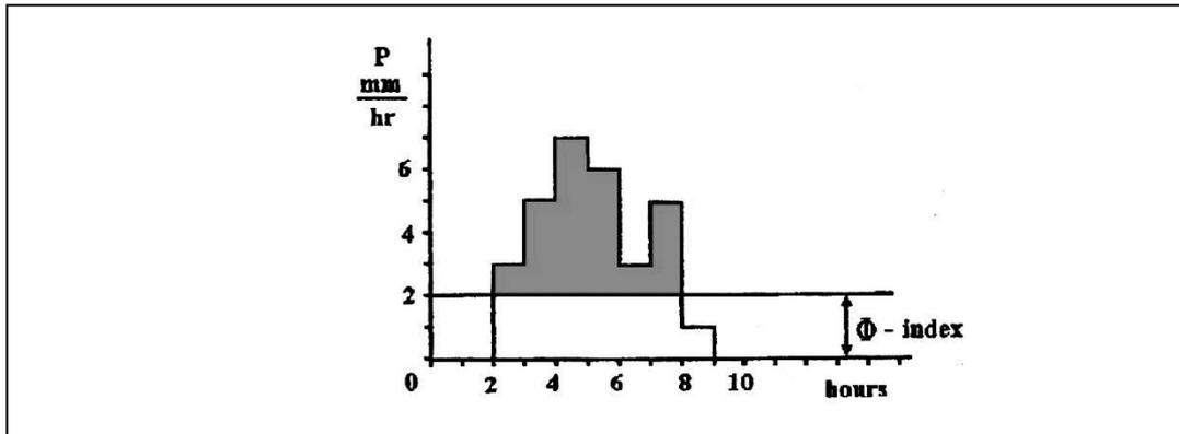
Figure 2.20: The  $\Phi$ -index to indicate losses
