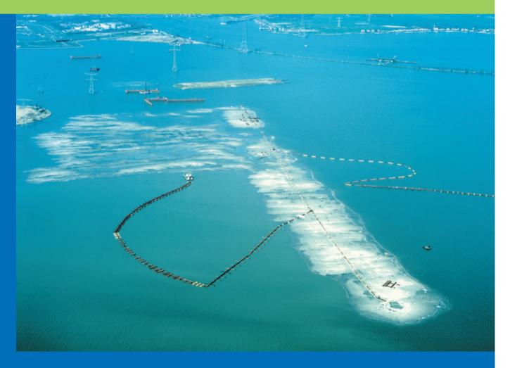
Betuwelijn, Netherlands: Detailed design of embankment construction for new railway line: geotechnical analysis for crossing areas with very soft subsoils and establishment of operational procedures within very strict environmental licenses.
