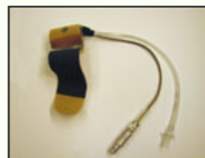
The finger cuff is used for the finger blood pressure measurement. A finger cuff contains an infrared LED (Light Emitting Diode) and a near-infrared plethysmograph, for the measurement of finger artery volume changes, and an inflatable airbladder, electrical shielding, and several layers of plastic and rubber with Velcro at the outside. A cuff cable connector and an air hose connector plug into the Frontend Unit. Cuffs are available in three sizes : small (white), medium (beige) and large (blue).
