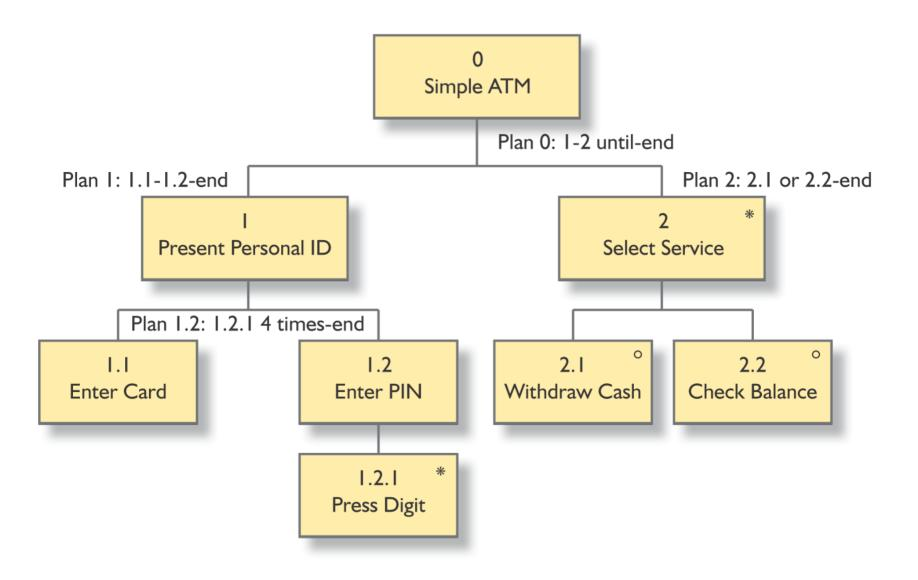
Figure 20.3 Hierarchical task model for a portion of an ATM.
