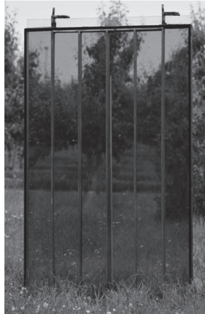
Fig. 04.58: The first 'Smart Skin' prototype with clear triple-layered glass, upside down.
