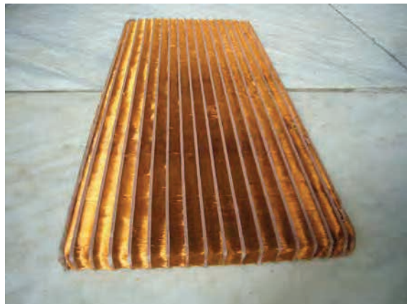
Fig. 04.30: Breathing Window fine-wire heat exchanger element: 7.5 km of 0.1 mm copper wires (400 g in total) run left to right; plastic partitions separate the canals where ingoing and outgoing air flows in turns exchange heat
