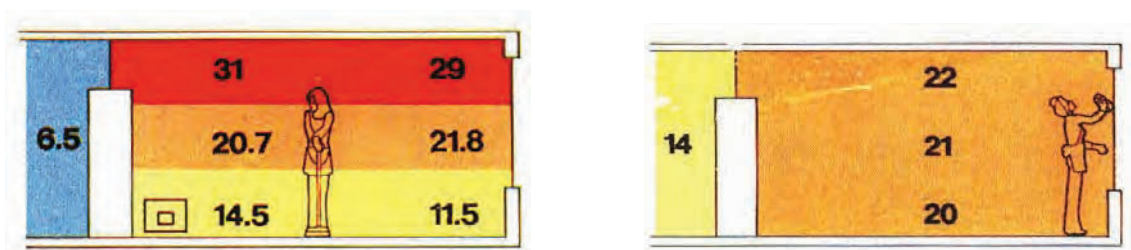
Fig. 04.24: Temperature distribution before (left) and after renovation (right)
