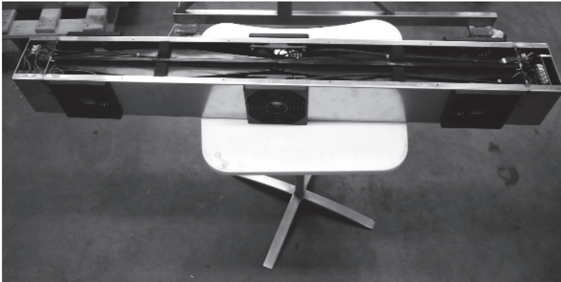
Fig. 04.36: The test version of a double Breathing Window: two Fiwihex elements in a compact box
