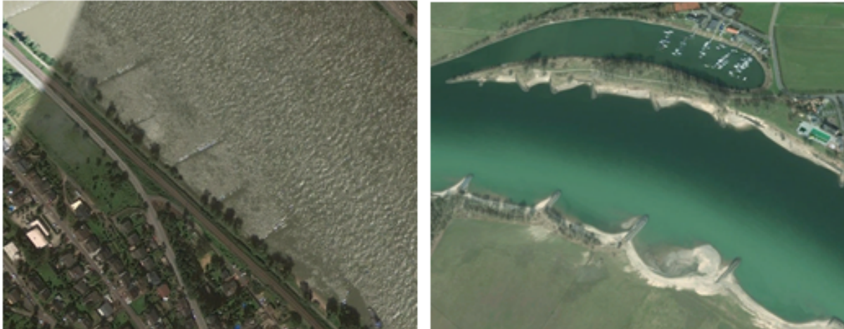
Figure A- 5 Groyne fields in Germany. Left: Submerged groynes in Trechtingshausen, Middle Rhine. Right: Emerged groynes near Wessel, Lower Rhine [Source: Google Earth].
