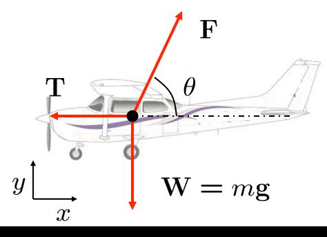
The plane is in static equilibrium Model as a particle and calculate: - Aerodynamic force  $\mathbf{F}$
