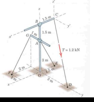
The tension T in the cable CD is equal to 1.2 kN.
