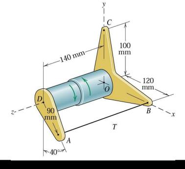
The shafts and attached brackets are twisted in opposite directions to maintain a tension **T** of 500 N in the wire joining A and B. Express the tension, considered as a force acting on A, as a vector and determine the projection of **T** onto the line DC.
