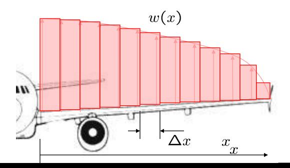
Magnitude of the equivalent force of a line distributed load
