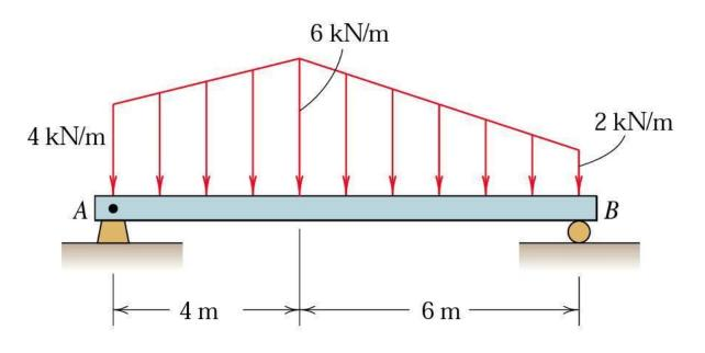
Determine the reactions at A and B for the beam subjected to the two linearly varying load distributions
