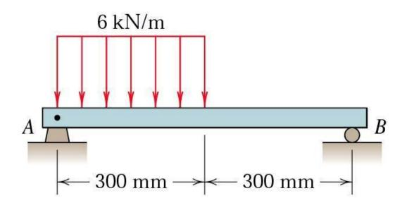
Determine the reactions at A and B for the beam subjected to the uniform load distribution
