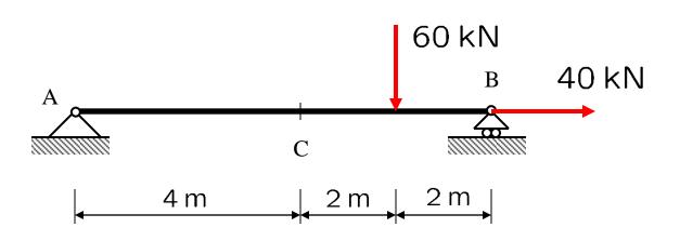
Calculate the internal forces in C.
