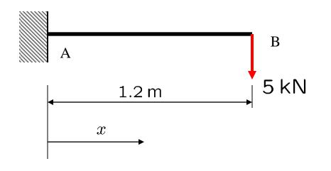
Determine the shear force and moment diagram of the cantilever beam.
