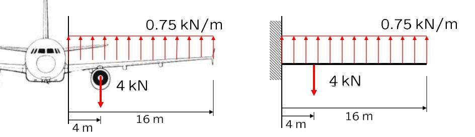
Determine the shear force and moment diagram of the wing of this airplane.
