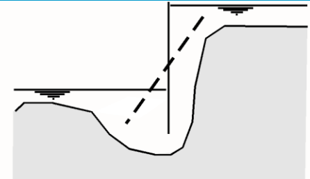
Phase 4 Complete piping and collapse
