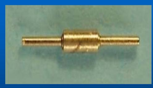
Check valve: - Ø 1.5 x 2.8 mm -  $\Delta P = 48 \text{ kPa}$ - Q ≥ 120.0 ltr/hr - m = 0.05 g
