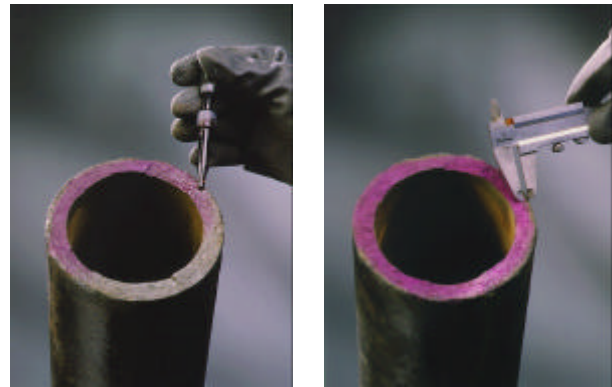
Fig. 12 - Phenolphthalein field test
