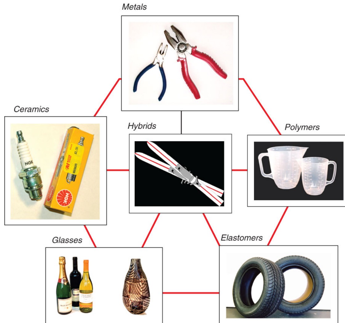
Figure 2.2 Examples of each material family. The arrangement follows the general pattern of Figure 2.1. The central hybrid here is a sandwich structure made by combining stiff, strong face sheets of aluminum with a low-density core of balsa wood.
