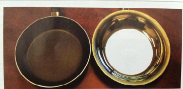
A quasicrystalline-coated pan (right) compared with a teflon-coated pan (left).
