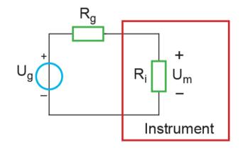
$$U_m = \frac{R_i}{R_g + R_i} U_g = \left(1 - \frac{R_g}{R_g + R_i}\right) \cdot U_g$$
