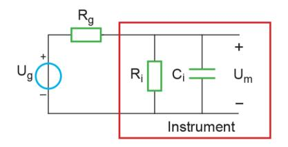
$$U_{m} = \frac{Z_{i}}{R_{g} + Z_{i}} U_{g} = \left(1 - \frac{R_{g}}{R_{g} + Z_{i}}\right) \cdot U_{g}$$
