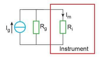
$$I_m = \frac{R_g}{R_g + R_i} I_g = \left(1 - \frac{R_i}{R_g + R_i}\right) \cdot I_g$$
