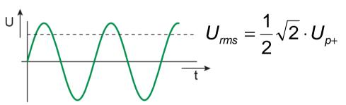
Correction factor is strongly dependent on the waveform!
