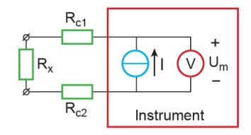
$$R_m = \frac{U_m}{I} = R_x + R_{c1} + R_{c2}$$
