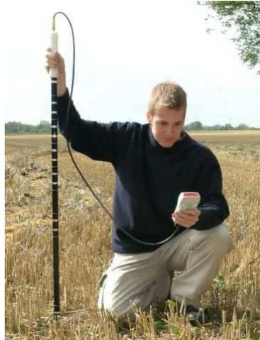
**Figure 2.14:** Frequency Domain Reflectometry (*PR2 Profile Probe - Delta-T Devices*)
