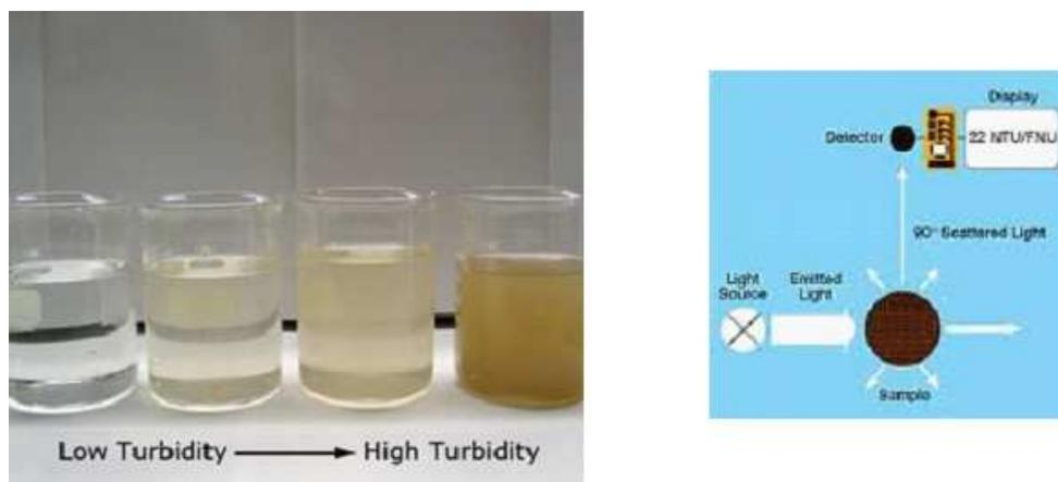
**Figure 4.23:** Principle of turbidity measurement
