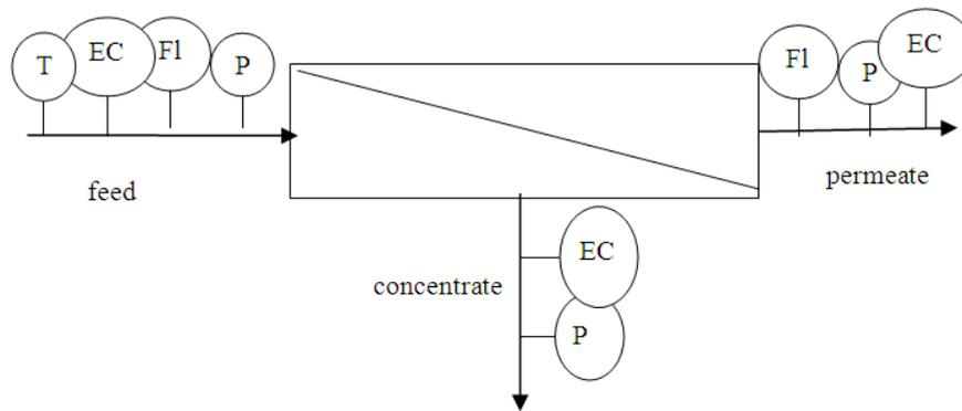
**Figure 4.20:** Monitoring equipment for the test rig
