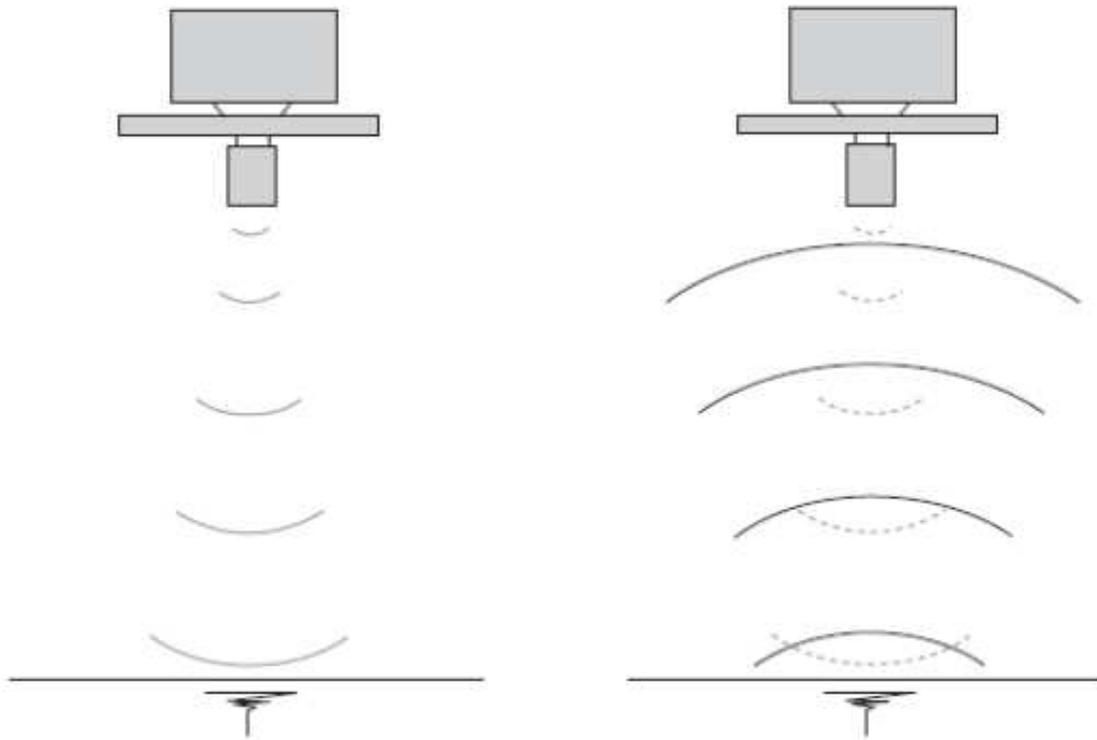
**Figure 4.2:** Principle of ultrasonic measurement: signal sending (left) and receiving (right) (RIONED [2009])
