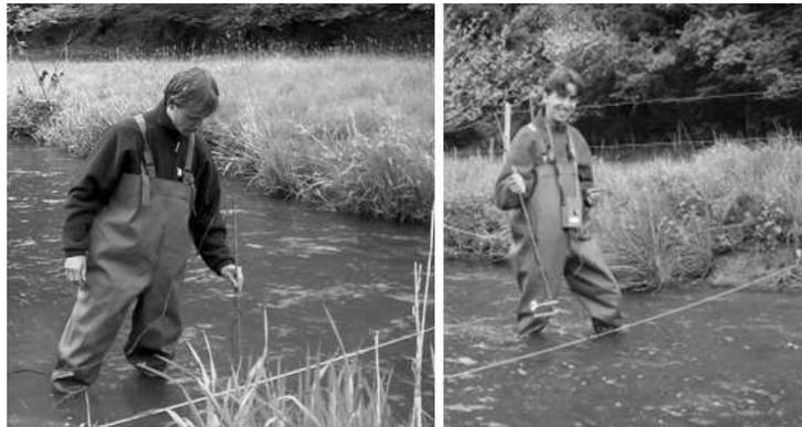
**Figure 2.18:** Measuring stream flow by wading
