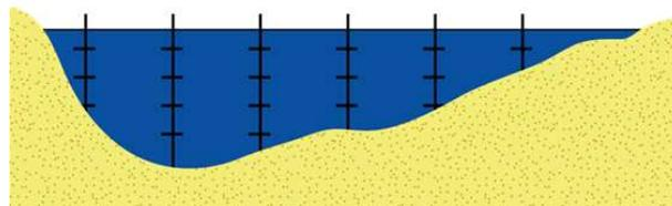
**Figure 2.16:** Example 'velocity-area-method'
