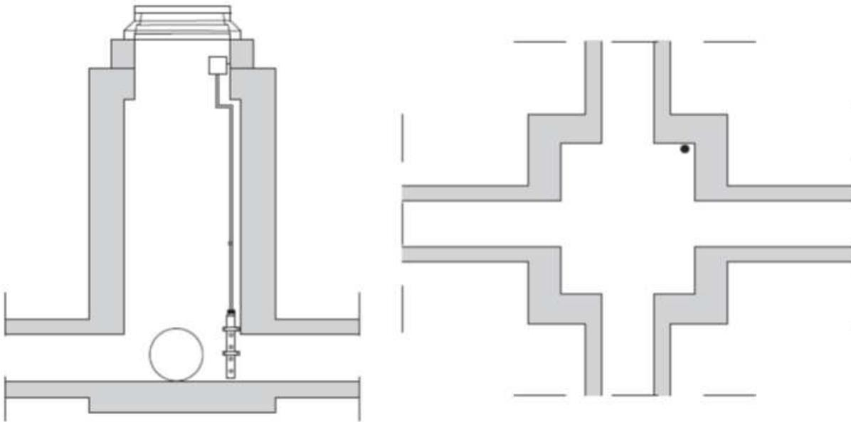
**Figure 4.4:** Position of pressure sensor in sewer manhole
