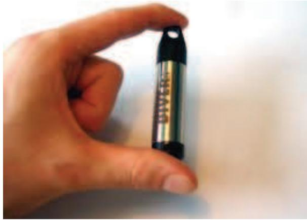
**Figure 2.15:** A pressure transducer used to measure groundwater heads
