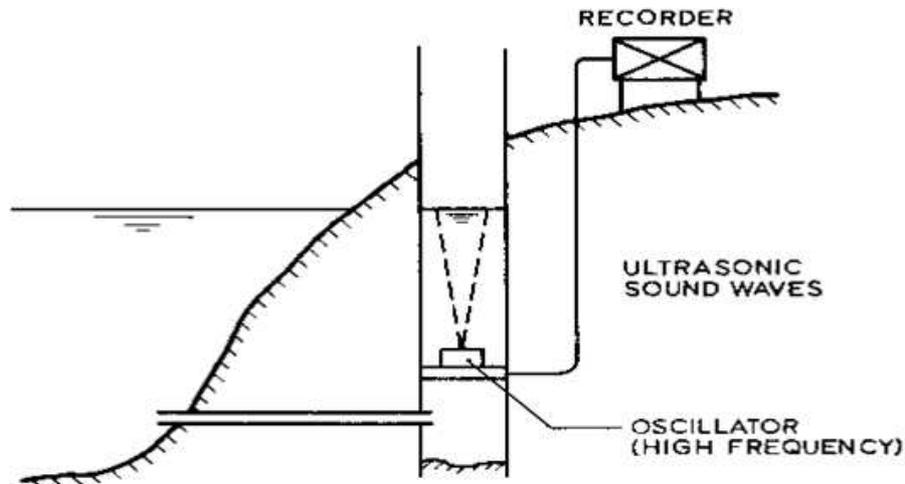
**Figure 2.24:** Ultrasonic water level gauge with sensor below the water surface
