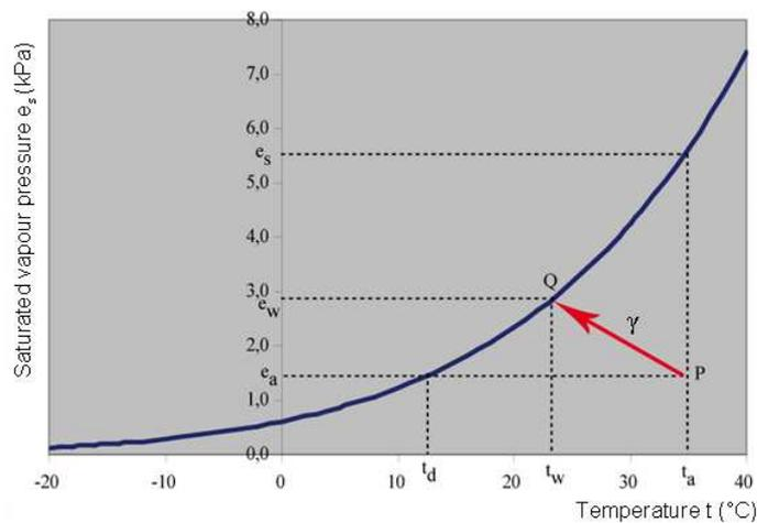
**Figure 2.6:** Saturation vapour pressure as a function of the air temperature
