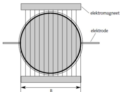
**Figure 4.9:** Principle of electromagnetic induction in a flow meter
