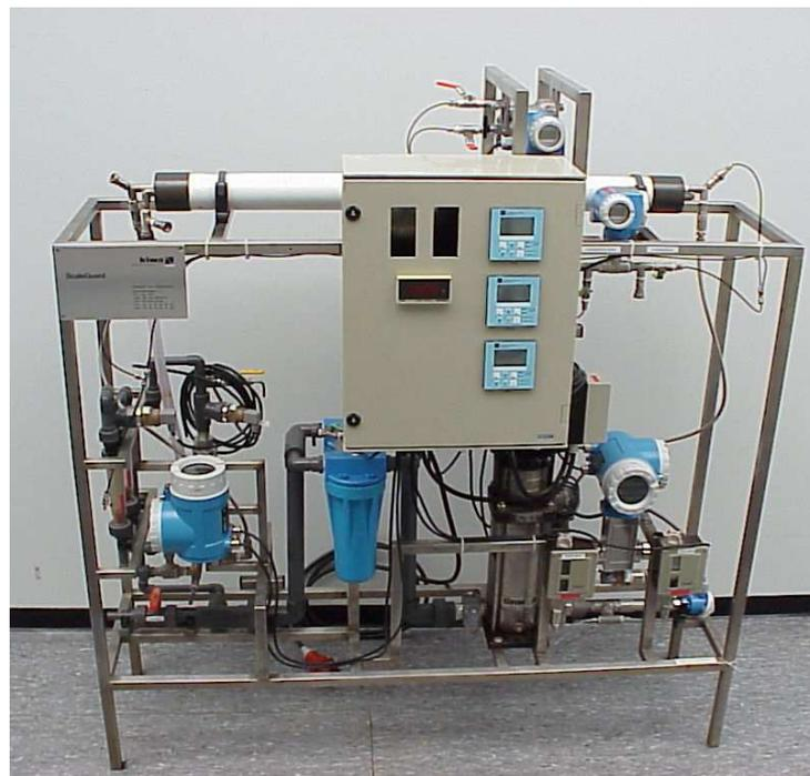
**Figure 4.19:** Test rig for nanofiltration or reverse osmosis
