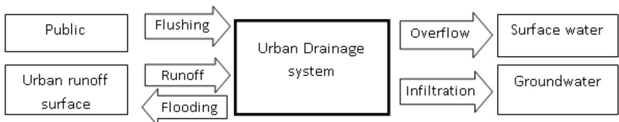
Figure 4.1: Interfaces between urban drainage system and urban environment
