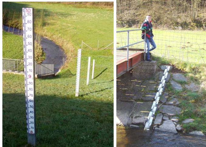
**Figure 2.23:** a) vertical staff gauge; b) inclined staff gauge
