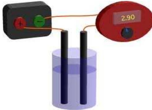
**Figure 4.22:** Electric conductivity (EC) measurement
