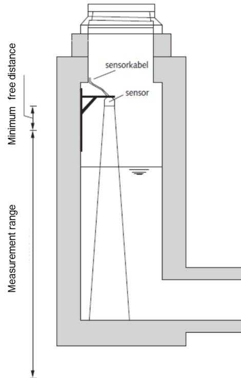
**Figure 4.3:** Installation of ultrasonic sensor in a sewer manhole. The measurement range covers only about 80% of the total possible water level variation. (RIONED [2009])
