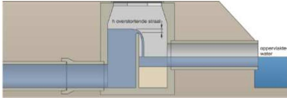
**Figure 4.5:** Principle of overflow weir constructed inside a sewer manhole. Water flows from the sewer system (left) over the weir towards surface water (right). (Courtesy of VPB)
