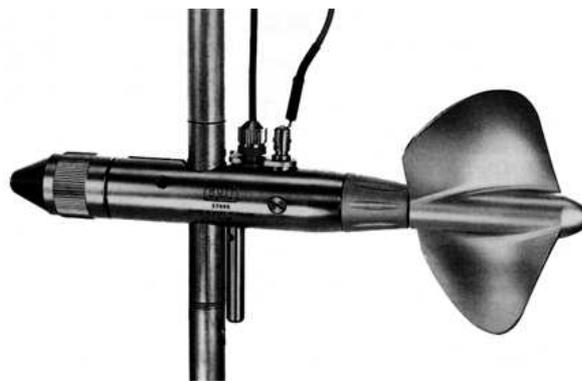
**Figure 2.17:** Propeller type current meter
