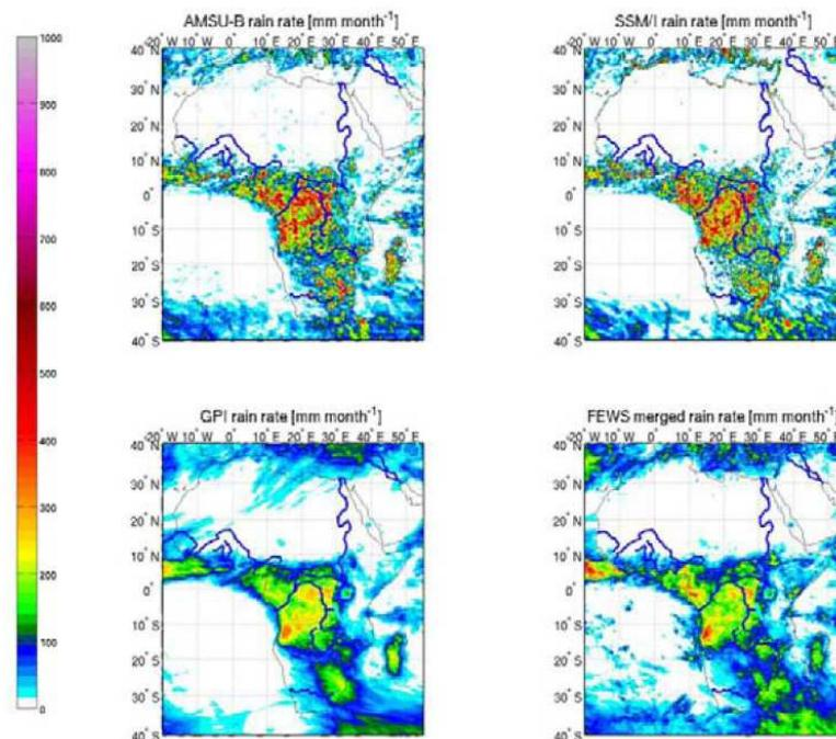
**Figure 2.4:** Three independent accumulated rainfall estimates and station data based estimates for a 30-day time window (November 1st until 30th 2007) over Africa. From left to right: AMSU-B microwave, SSM/I microwave, Meteosat GPI, and a merged estimate. The merged estimate shows the impact of rain gauges, especially over the Atlantic Ocean.
