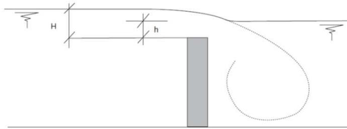
**Figure 4.6:** Flow over a drowned weir: the discharge over the weir is influenced by the downstream water level, which negatively affects the accuracy of discharge measurement over the weir.
