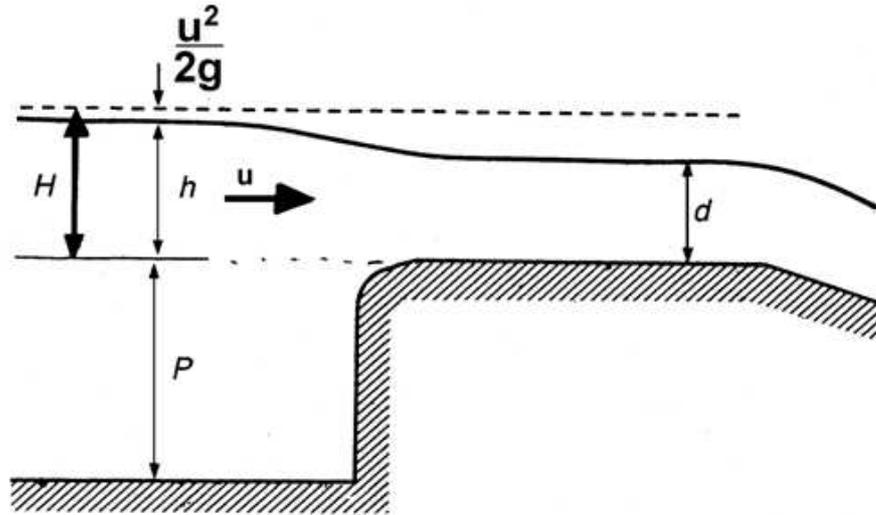
**Figure 2.26:** Schematic illustration of principle and theory of flow over broad crested weir
