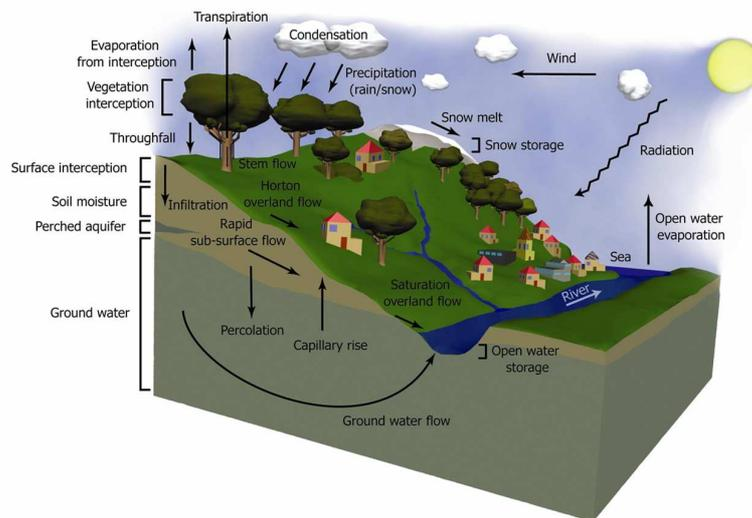
**Figure 2.1:** The hydrological cycle.
