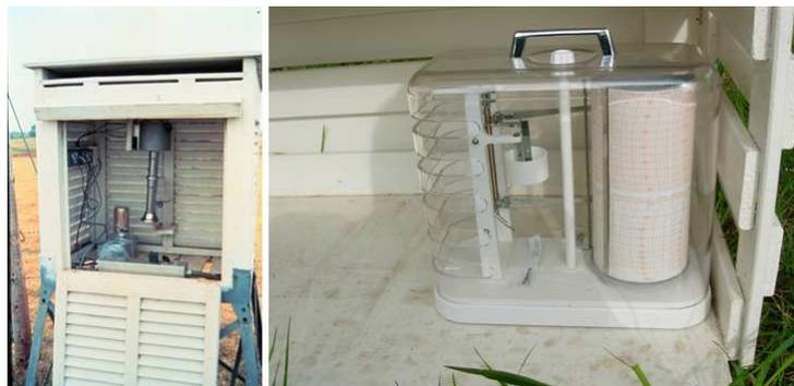
**Figure 2.7:** Stevenson Shelter with combined hygrometer and temperature meter
