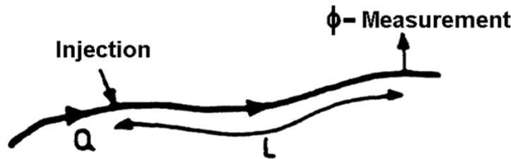
Figure 2.22: Dilution gauging for reach L
