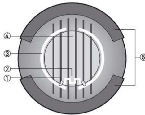
**Figure 4.10:** Principle of electromagnetic flow meter for part-full pipe: 1- Electrodes, 2- Induced voltage (proportional to flow velocity), 3-Capacitive plates in liner for height measurement, 4-Magnetic field, 5-Field coils
