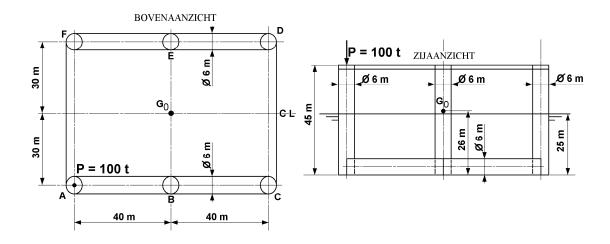
Figure 0.5: Loading a Drill Platform
