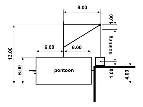
Figure 0.4: Lift Operation by a Pontoon
