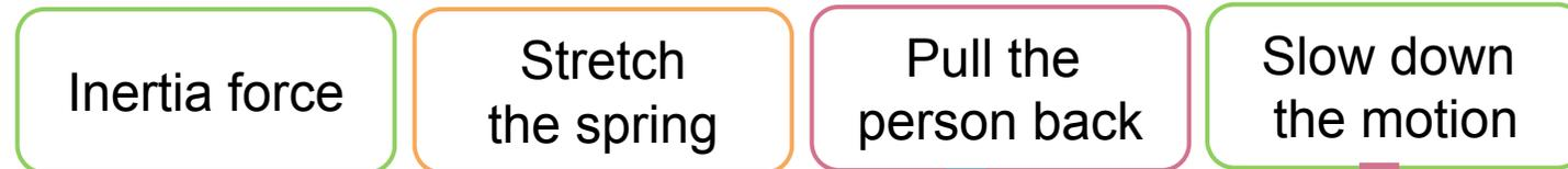
$$-m \frac{dx^2(t)}{dt^2} + mg - k \begin{cases} 0 & x(t) \leq L \\ x(t) - L & x(t) > L \end{cases} - \text{signum}\left(\frac{dx(t)}{dt}\right) \frac{1}{2} \rho_{air} A c_d \left(\frac{dx(t)}{dt}\right)^2 = 0$$
