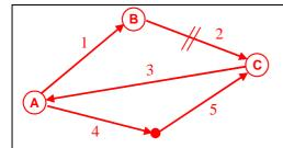
Only travellers from A to C have a choice of route (route 1 consisting of links 1 and 2, and route 2 consisting of links 4 and 5), all other travellers only have a single route to choose from. Let AB be the number of travellers from A to B, CB from C to B, etc. Let AC1 be the number of travellers from A to C choosing route 1, and let AC2 be the number of travellers from A to C choosing route 2.
