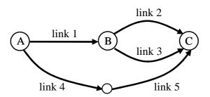
Each link in the network is assumed identical and the travel time on each link *a* is given by  $t_a$ .
