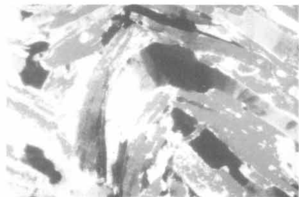
Figure 7-18: Micrograph of deformed quartz-mica schist. See exercise 7-6.
