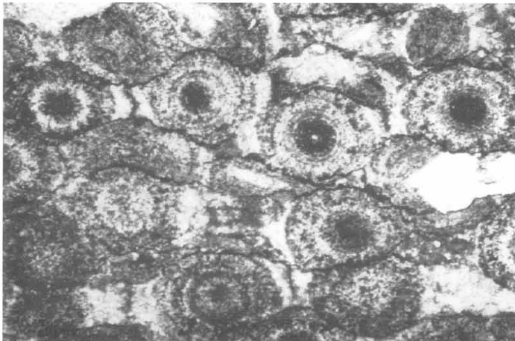
Figure 7-7b: Thin section of stylolite seams eroding ooids of oolitic limestone, accommodating vertical shortening of the rock volume.
