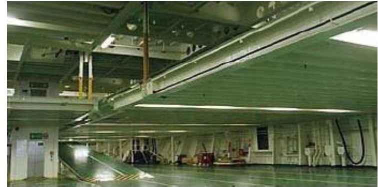
Hoistable car decks
