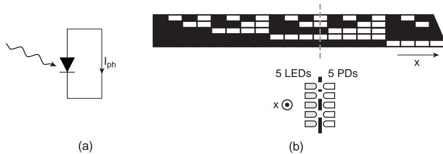
Figure 2.2, (a) The photodiode is a self-generating sensor and (b) the 5-bit linear encoder is an example of a modulating sensor with five Light Emitting Diodes (LEDs) as the light sources and five Photo Diodes (PDs) as the detectors.
