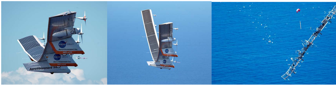
Figure 1.6 Illustration of the difference between stiffness and strength; the flexibility of the wings relates to stiffness (low stiffness gives significant wing bending), whereas strength relates to final failure of the structure
