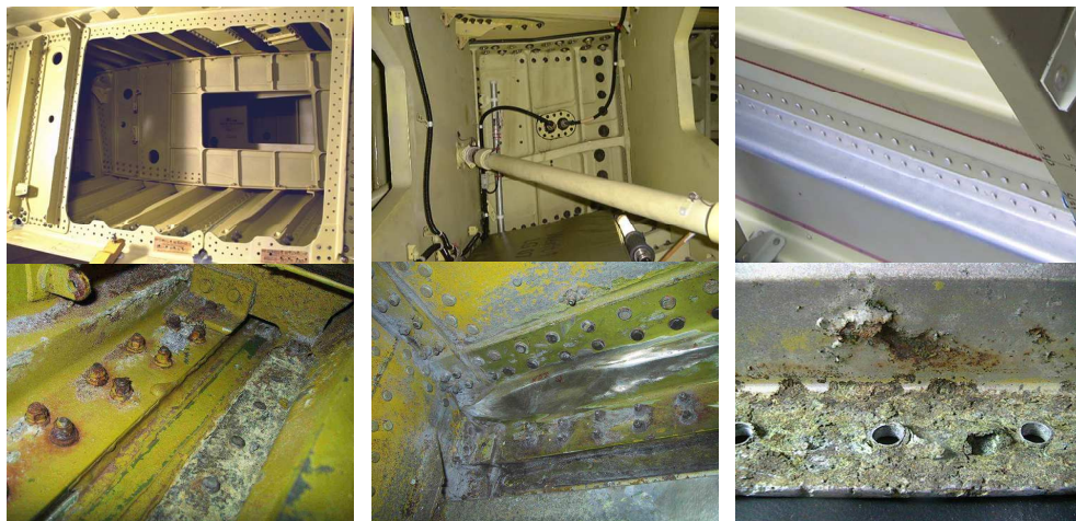
Figure 2.12 Examples of brand new virgin structures (upper row) and structures after decades of operational use (lower row)
