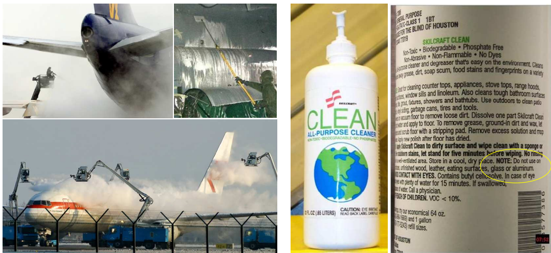
Figure 2.11 Photos of de-icing and cleaning procedures (left) and an example of cleaning agent inappropriate for aluminium (right)
