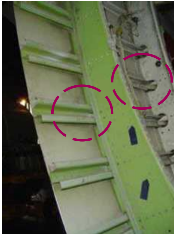
Figure 5.31 Illustration of intersections between frames and stringers in a fuselage panel
