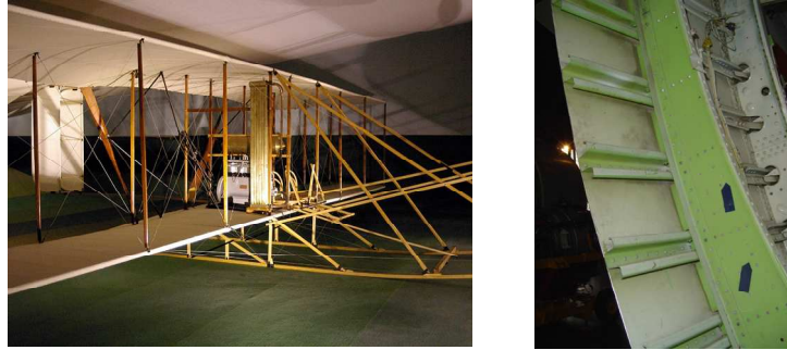
Figure 8.6 Illustration of the different design related to material usage; wood, linen and steel trusses (left) and load bearing stiffened aluminium shell structure
