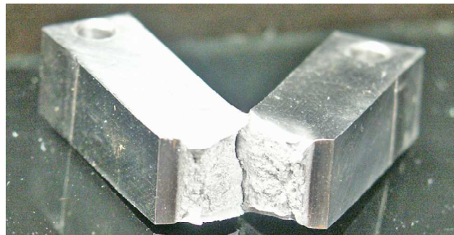
Figure 1.19 Test set-up for impact toughness measurements (left) and a fractured impact toughness specimen (right).
