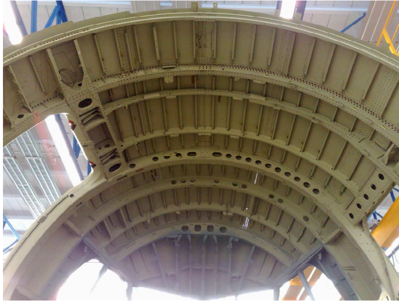
Figure 5.3 Photo of the shell structure of the cockpit section of the Fokker 100 aircraft (component located in the collection of the Structures & Materials Laboratory)
