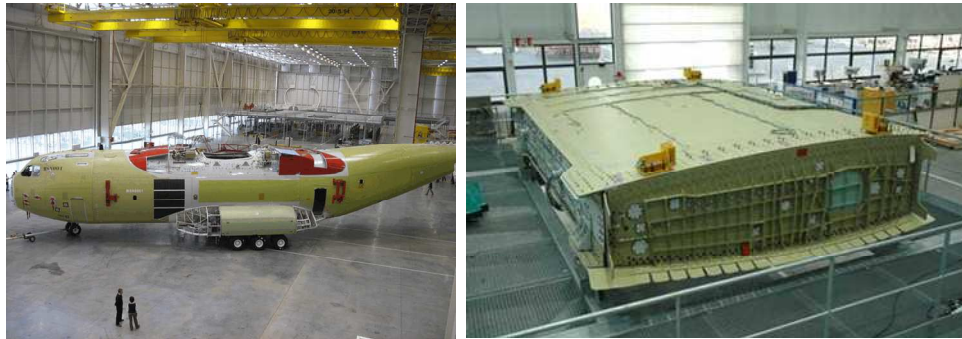
Figure 6.14 A400M transport aircraft in production (left) and the centre wing box (right)
