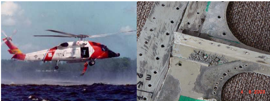
Figure 2.8 Illustration of a humid and salty environment (left) and the consequence of corrosion for an aluminium structure (right)
