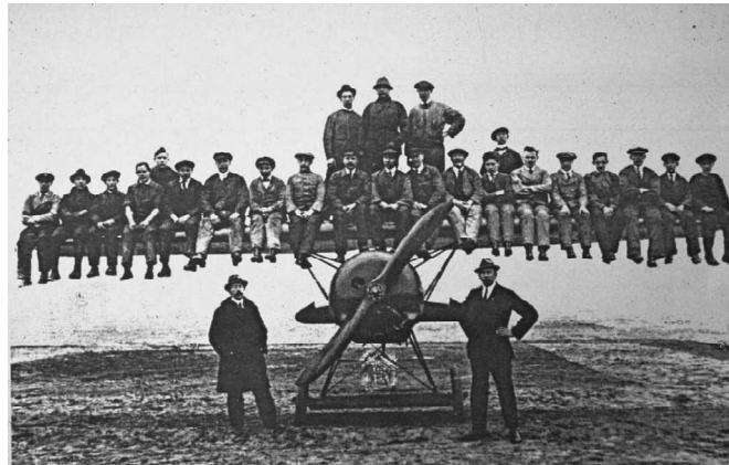
Figure 9.3 Illustration of a typical static strength tests on early aircraft
