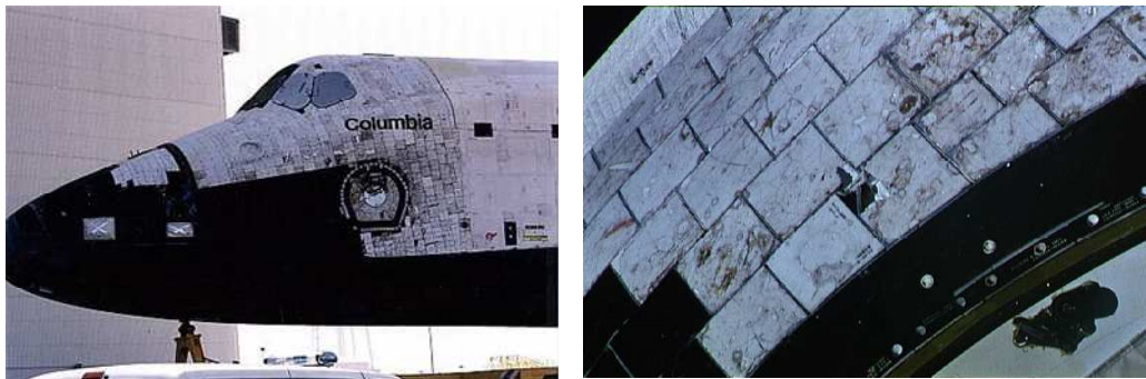
Figure 2.9 Illustration of surface of the Space shuttle (left) and the consequence of the aggressive environment on the structure's surface (right)
