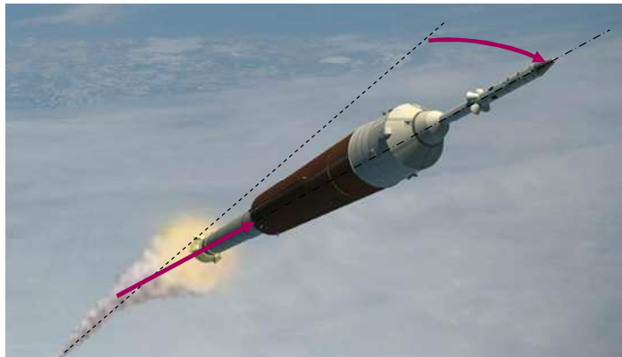
Figure 6.17 Illustration of the axial and lateral loads and movements
