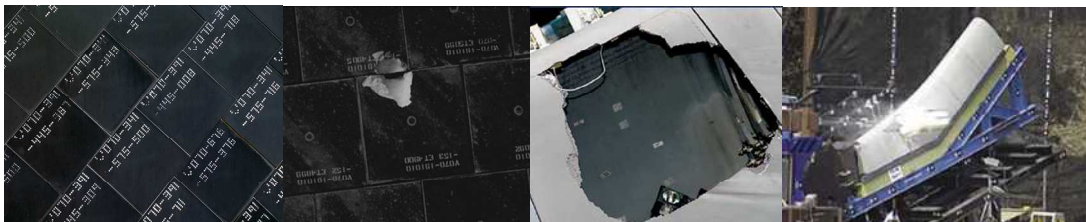
Figure 3.8 Image of the ceramic tiles with an impact (left) and debris from the accident (right)
