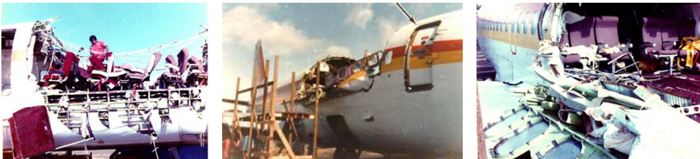
Figure 9.7 Photos of the damage to the fuselage of the Aloha airlines aircraft
