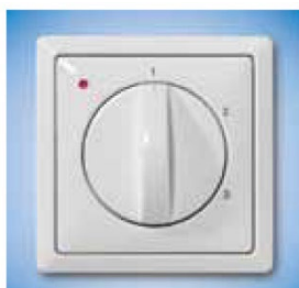
Fig 3.1. Three-position switch for a balanced ventilation system with a filter indicator light on the left. This red LED switches on when the filters need cleaning. It's a simple feature that ensures that residents are well informed and will clean or replace the filters on time. Photo: Brink Climate Systems
