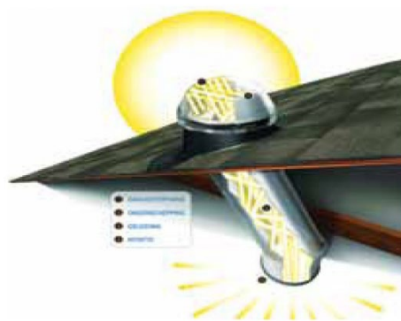
Fig. 1.15: A 'light tube' or 'roof light spot' can be useful to provide built-in or long rooms with (more) daylight when a skylight or sky dome is not possible. The tube is internally equipped with a highly reflective material. There are several manufacturers who provide these daylight tubes.
