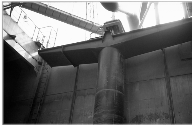
Figure 2-101 Adjustable overflow over the full width of the hopper
