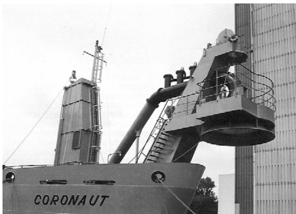
Figure 2-10 Pump ashore connection
