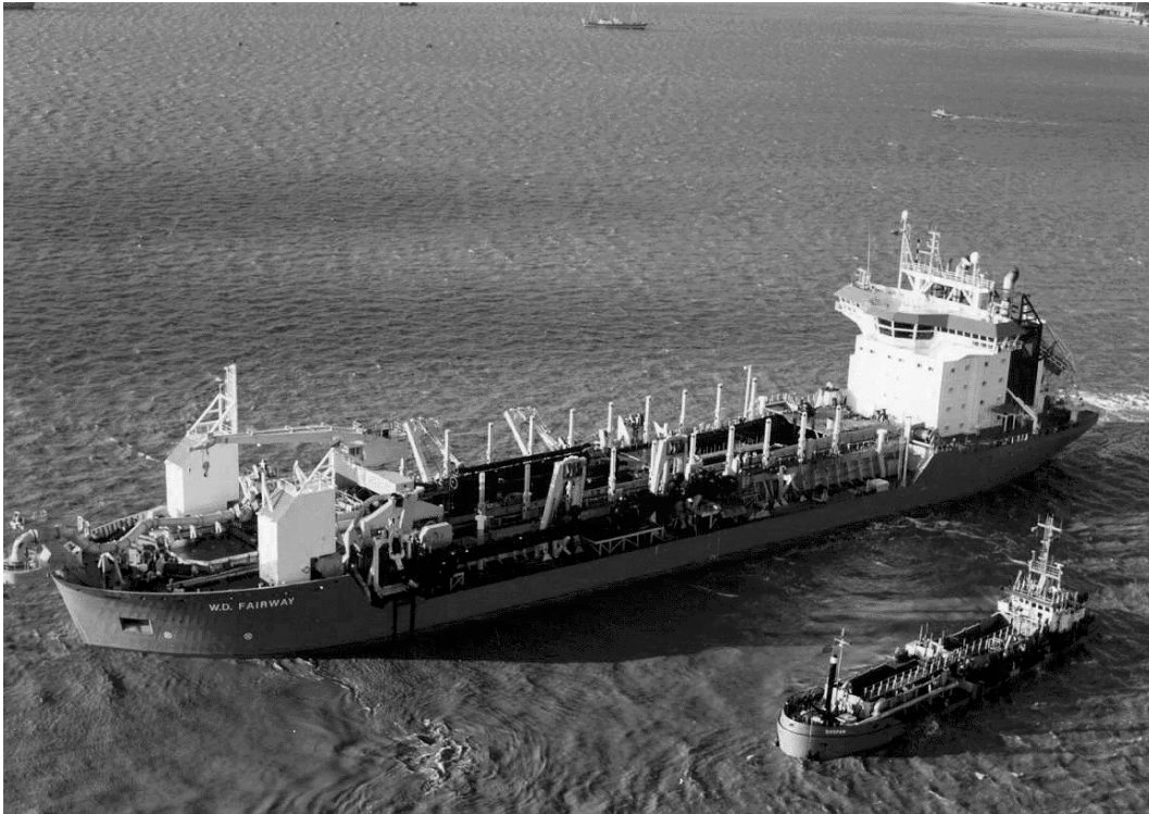
Figure 2-14 Different scales Fairway (23.347 m 3 ) and the Sospan (700 m 3 )
