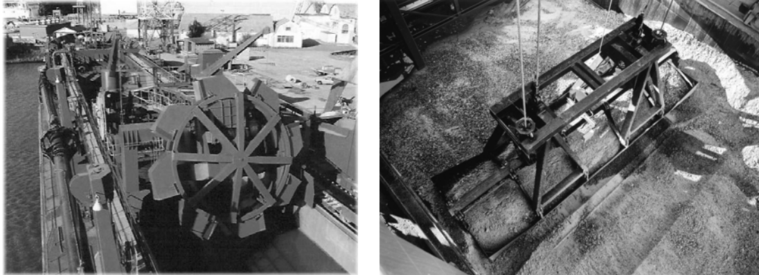
Figure 2-114 Dredging wheel unloader (Left) and clamshell unloader (right)
