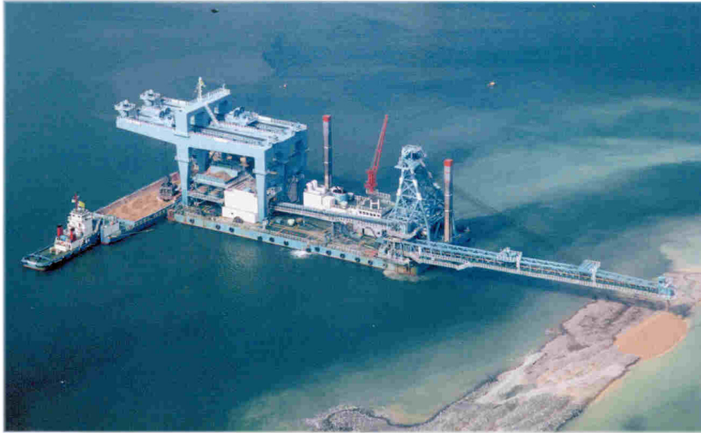
Figure 7- 3 Grab bucket reclaimer
