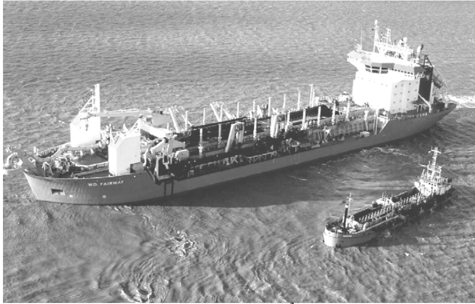
A 23350 and 700 m 3 hopper dredger
