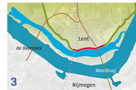
An ancillary channel is to be dug in order to give the river more room. This will create an elongated island.
