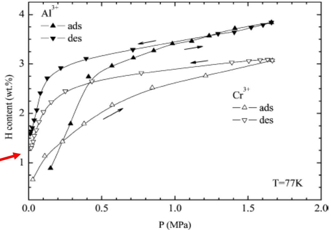
Fig. 2 PCI curves (▲: adsorption; ▼: desorption) measured at 77 K up to 1.6 MPa of hydrogen pressure for the MIL-53 samples with M = Cr<sup>3+</sup> (open symbol) and M = Al<sup>3+</sup> (full symbol).
