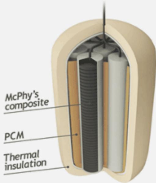
A patented Phase Change Material (PCM) brought into thermal contact through the metal walls with the McPhy composite allows to store heat energy during loading and to return it during unloading.
