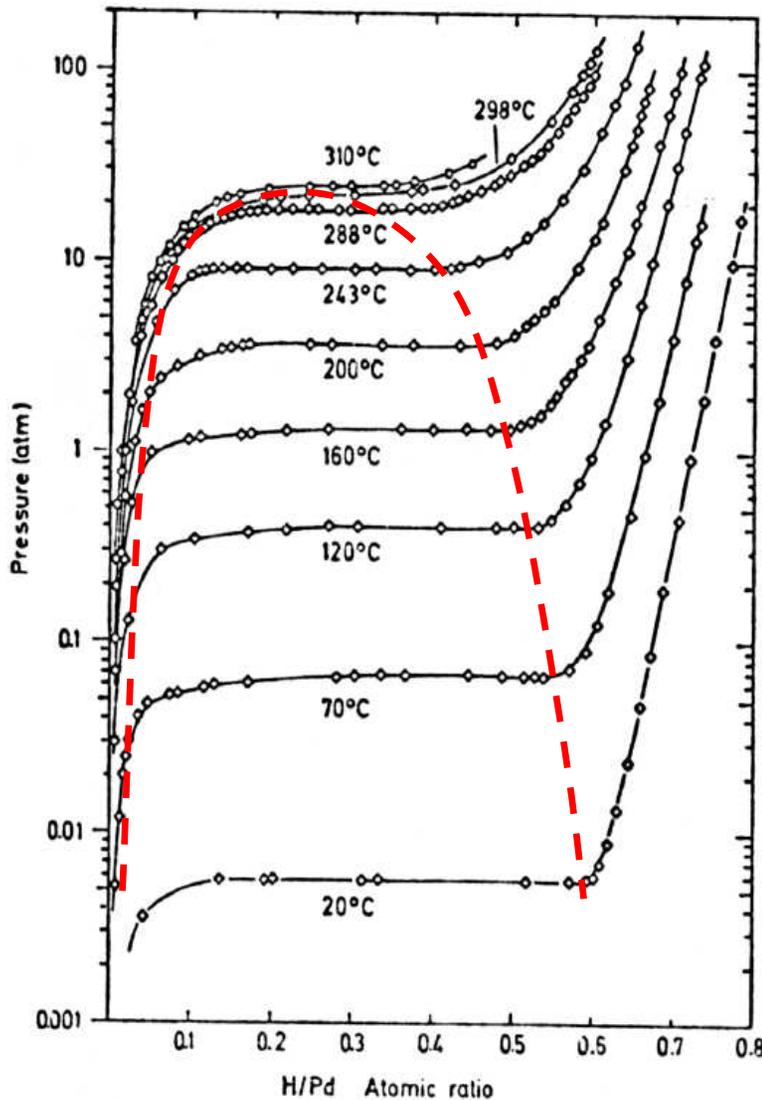
$\alpha$  is a H-poor phase,  $\alpha'$  a H rich phase. Below the parabola they occur next to each other.
