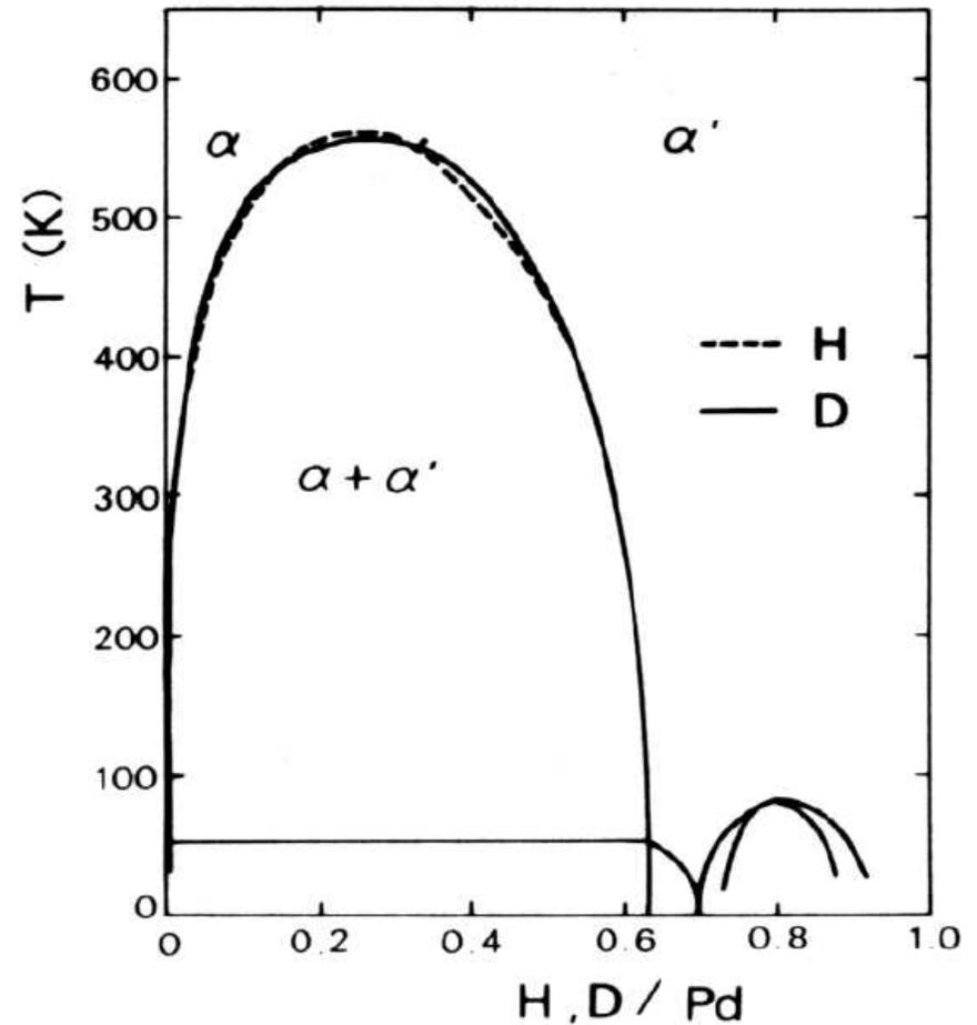
The reason for the phase separation into 2 phases is the same as for Li-insertion compounds (see batteries)
