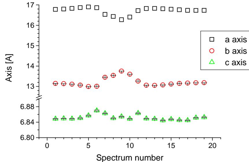
Most remarkable result: the loading with hydrogen causes the lattice Parameters to change a lot, up to 7%. This was not observed before for Hydrogen.
