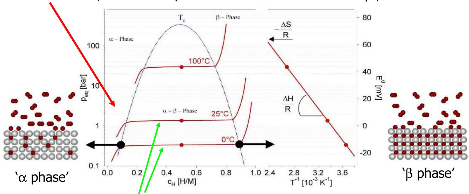
Here there is equilibrium between gas,  $\alpha$ , and hydride  $\beta$  phase. The  $\alpha$  phase corresponds to the normal metal with some dissolved H in it, but too little to form the real hydride.
