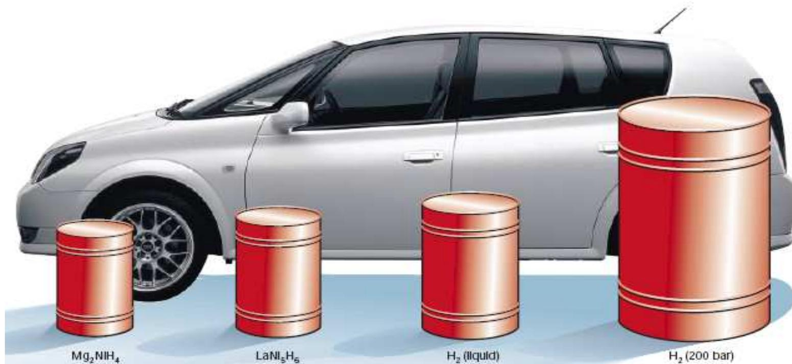
Metal hydrides can have higher volumetric H densities than liquid  $H_2$
