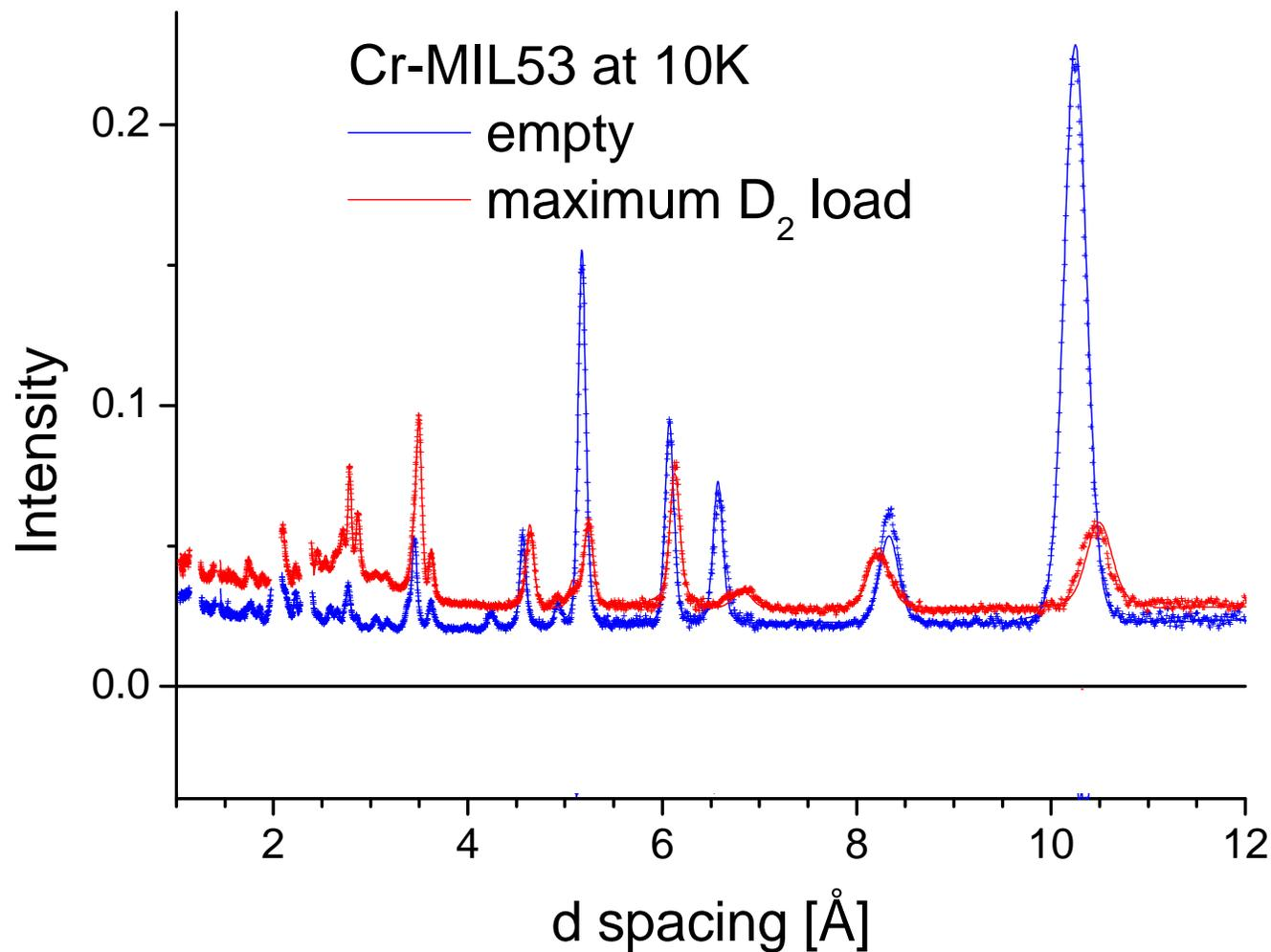
Large change of neutron diffraction pattern when D<sub>2</sub> is loaded.
