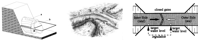
Fig. 469 The oldest one way sluice found in the Netherlands and its modern principle b
