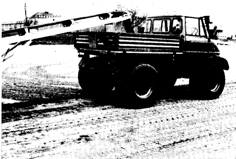
Fig. 4.16 Wheeled dumper with oversized low pressure pneumatic tires
