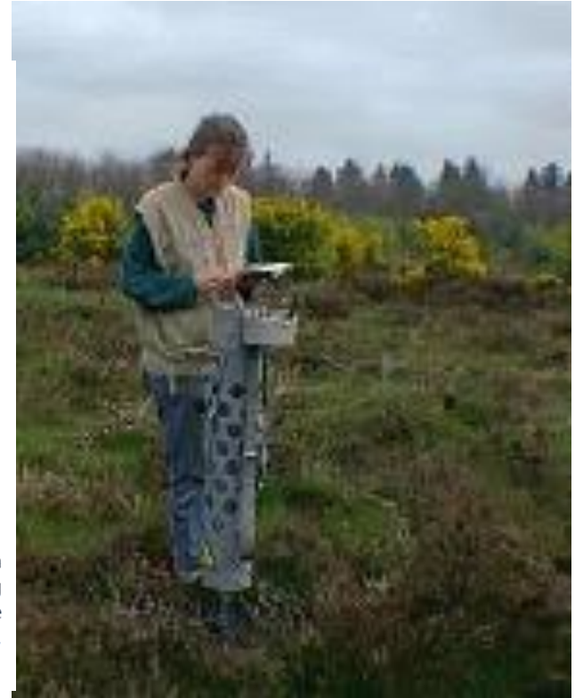
Fig. 6.2. Components of a portable neutron soil-moisture meter, including a probe (with a source of fast neutrons and a detector of slow neutrons) lowered from a shield containing hydrogenous material (e.g., paraffin, polyethylene) into the soil via an access tube. A scaler-rate meter is shown alongside the probe. Recent models incorporate the scaler into the shield body, and the integrated unit is lightweight for easy portability.
