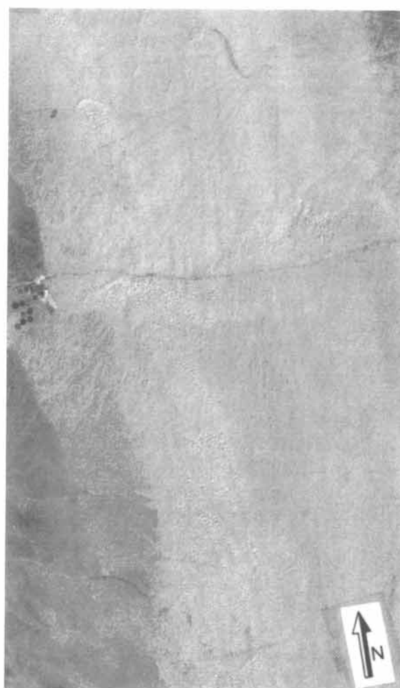
Figure 16-27b: Landsat MSS image across same area portrayed in Figure 16-27a shows bedrock structures are entirely obscured by Ad Dhana sand sea. Thin E-W line in image is railway track.
