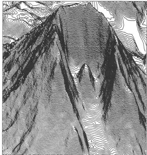
Figure 17-4: Perspective landscape of Mount St. Helens, processed from elevation-data files (DEM), using GRIDZO.
