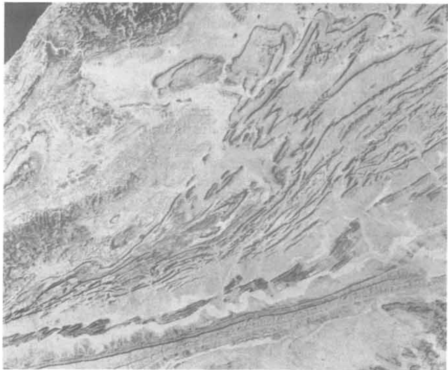
Figure 16-19a: Part of Landsat MSS of dextral Moroccan Border fault, separating Tindouf basin of the Draa Plateau to the south from tightly folded Devonian limestone and sandstone in the north wall.
