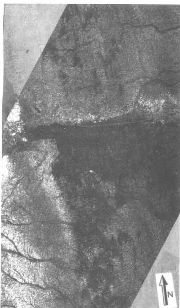
Figure 16-27a: L-Band radar image, collected by Space Shuttle Endeavour from Wadi Sahba area, Saudi Arabia. The trace of the E-W trending Sahba fault is clearly visible. Image width is 40 kilometers.
