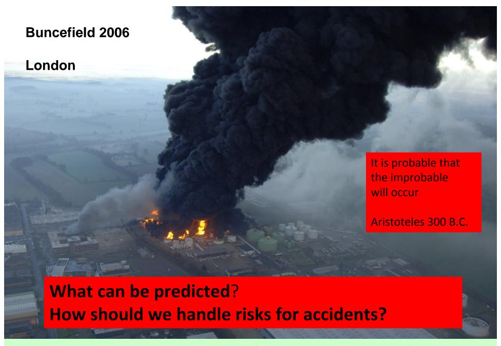
Overfilling of tank 912 led to an escape of fuel (now known to be unleaded petrol); and how this in turn led to the formation of a cloud of flammable vapour that subsequently ignited
