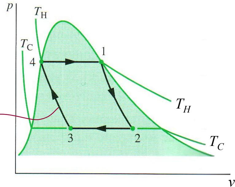
The compression of a two-phase system has (technical) disadvantages and power-cycles with full condensation will later be discussed
