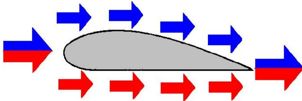
Since the pressure is higher beneath the wing the wing is pushed upwards.
