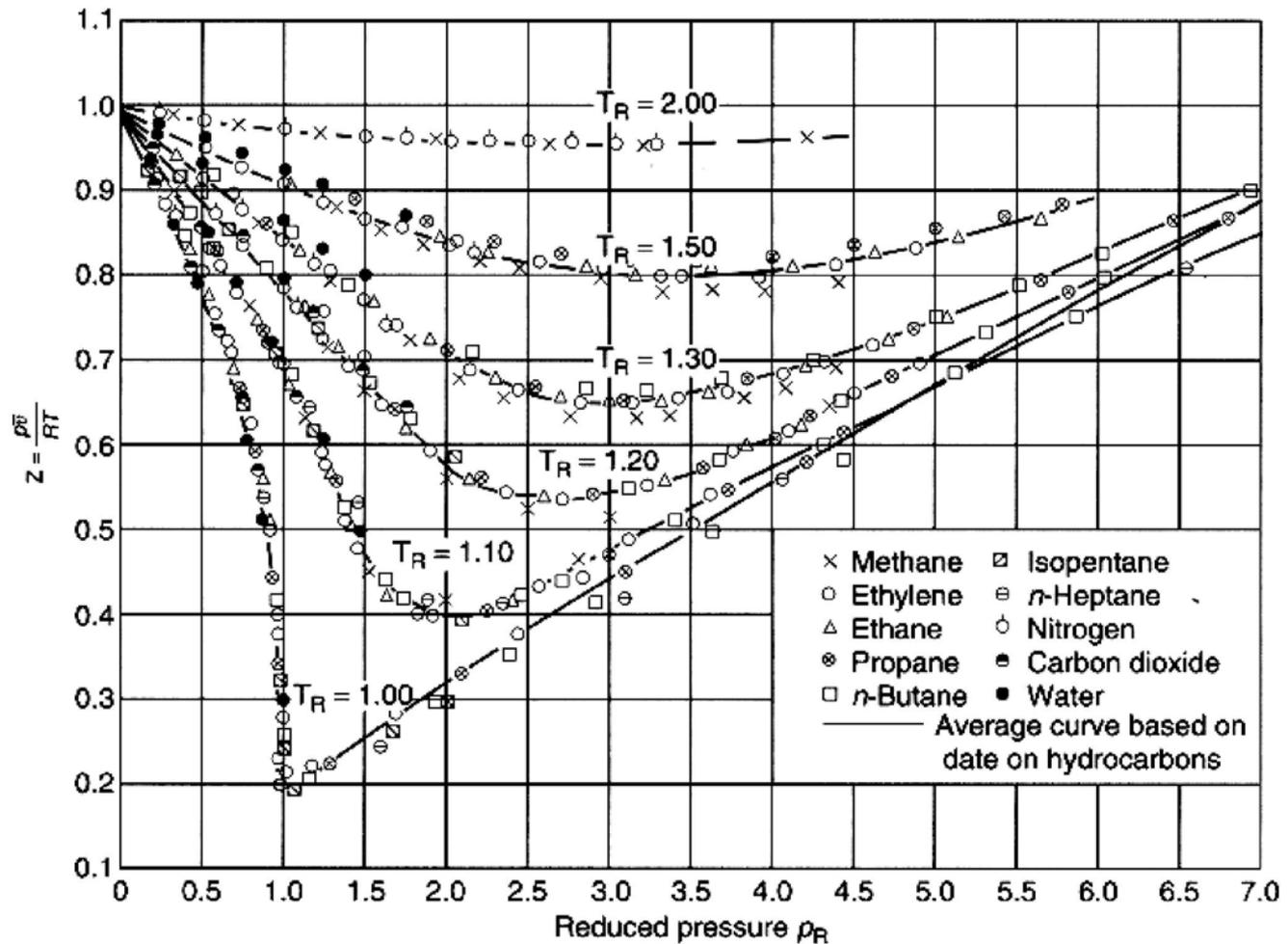
Figure 3.11 Generalized compressibility chart for various gases
