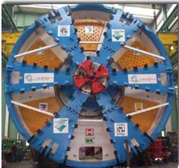
Bore head Westerschelde Tunne D= 11,33 m
