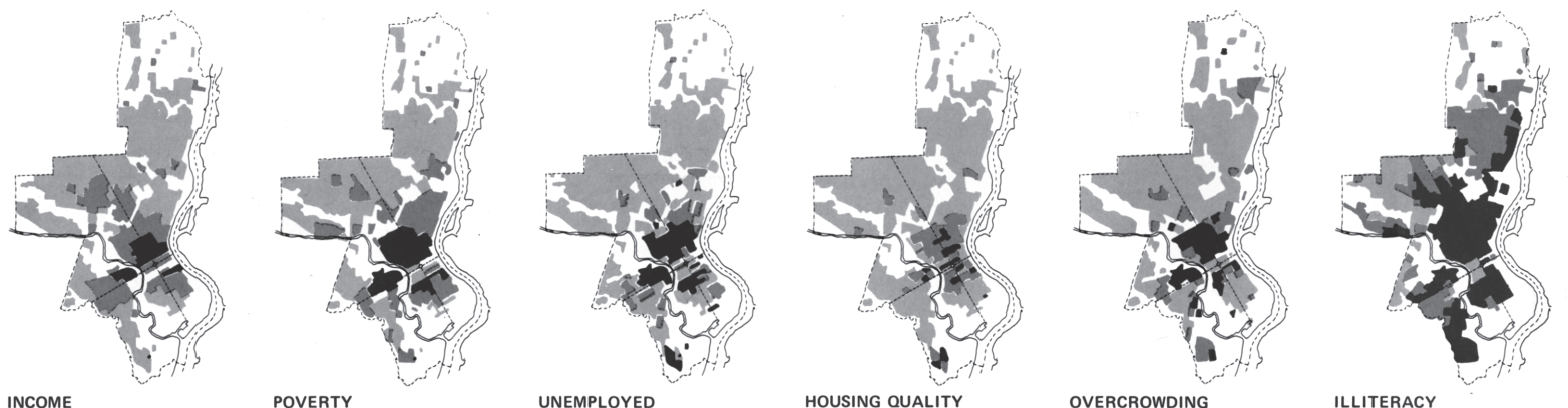
38 Sieve analysis according to McHarg (1969)
