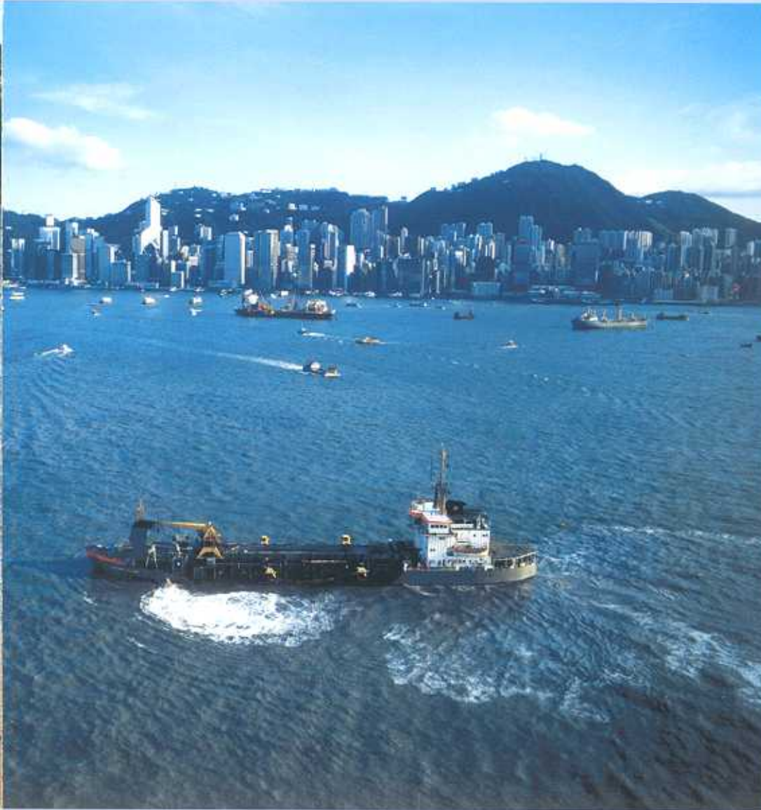
A Trailing Suction Hopper Dredger working in Hong Kong waters for the construction of the Yau Ma Tei Reclamation,
