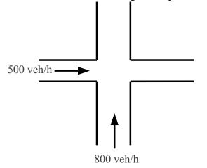
(a) What is the fraction of time traffic is flowing over the stop line per direction as (2) function of the cycle time c?
