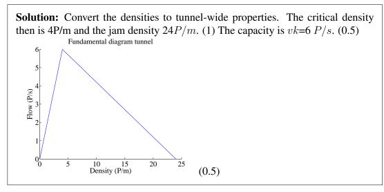
Between 11-12 am, the average flow through the tunnel is q = 180 P/min.
