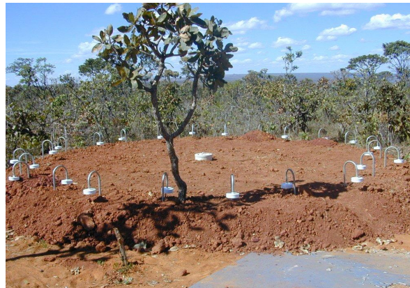
Figure 1.2: An array element with its noise reducer (IS49, Tristan da Cunha (left) and IS09 Brasilia (right)). The microbarometer is located in the vault in the center of the picture. The noise reducer consists of pipes with discrete inlets. Typical sizes are 20 to 70 meter depending on the expected wind speeds.
