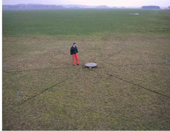
Figure 1.2: A noise reducer as applied in the Netherlands on Air Force Base Deelen. The system consists of six porous hoses of 7 meters length. The porous hose is commercially available as soaker hose.
