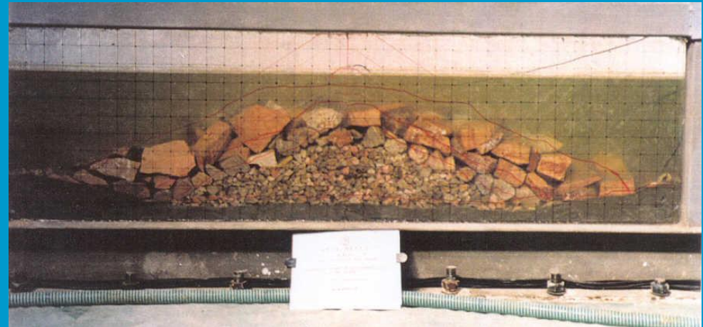
Failure of breakwater by earthquake
