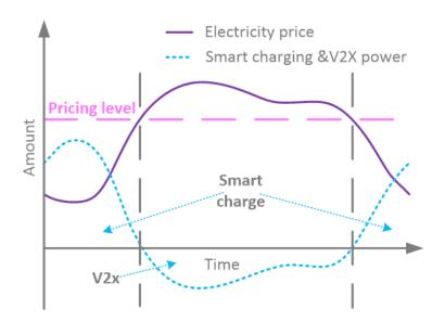
The charging power is increased when the electricity price is low, and the charging power is decreased or even stopped when the electricity price is high. Further, customers can get more profit when the V2x is applied. For example, we can charge the cars when the electricity is cheap and discharge the car via V2x when electricity is expensive and above a certain pricing level. In this case, the "x" of the "V2x" can be home, building or the grid.
