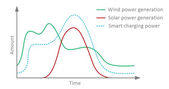
Smart charging can help in controlling the charging power of the car based on the renewable energy production, say from solar and wind generators. Further, with V2G, the electric cars can be used as massive energy storage to balance the variable generation from renewable energy sources.
