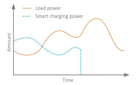
The first load balancing approach is to shift the charging time slot and to adjust the charging power based on the grid capacity and local loading condition. For example, when the load on the grid is low, the EV charging power can be increased. Alternately, if the load power increases, then the EV charging power can be subsequently reduced. Finally, the EV charging can be stopped if the grid is overloaded and remain so until the load power is back to normal.
