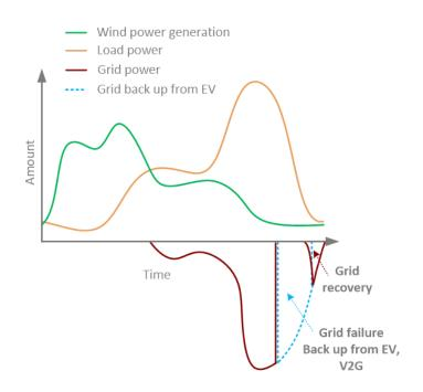
In the future, electric vehicles can even operate as a backup for the grid on a relatively large scale. In case of a short duration failure, EVs can be connected to the grid, to our homes or to loads and can be controlled to provide emergency power via V2G.
