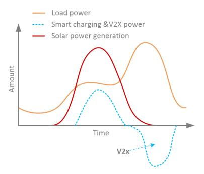
Here, the aggregated EVs can work as mass storage in the grid. With controlled charging, the EVs can be charged when there is extra renewable energy generation, and they can discharge via V2G to feed the grid when is a peak load in the evening. By doing so, the peak of both generation and consumption can be shifted, and the electric power demand-supply gap can be perfectly matched.
