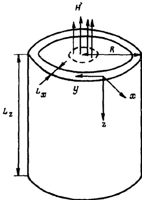
Lithium film evaporated on a quartz filament
