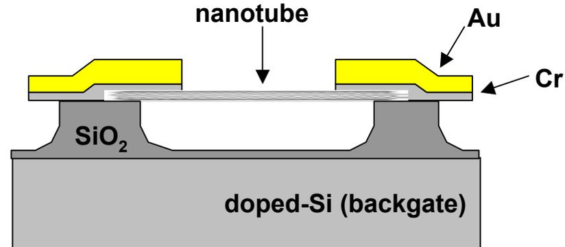
nanotube with diameter,  $r$ , above a ground plane at distance  $h$ :  $C_{\text{NT}} = \epsilon_0 \epsilon_r 2 \pi L / \ln(2h/r)$
