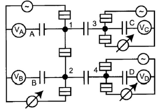
**Experiment:** SETs 3 and 4 work as electrometers to measure charges at the islands 1 and 2
