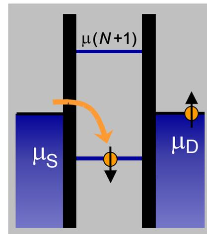
inelastic co-tunneling: excitation spectrum
