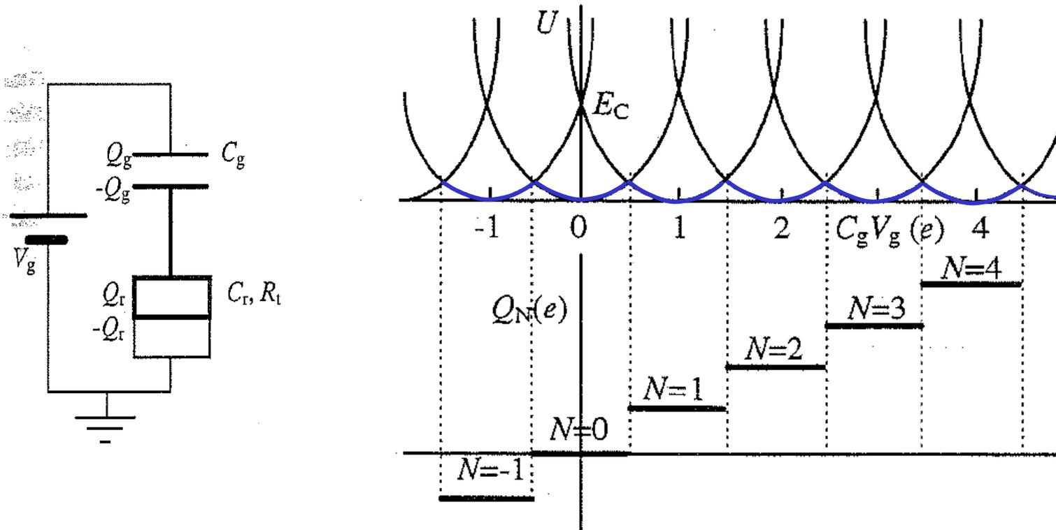
We take as a reference configuration the one for which all voltages and the charge are zero. The electrostatic energy with respect to this reference configuration after changing the source, drain and gate potentials and putting  $N$  electrons (of charge  $-e$ ) on the island is then found as the work needed to put this extra charge on the island and the energy cost involved in changing the external potential when a charge  $Q$  is present:
