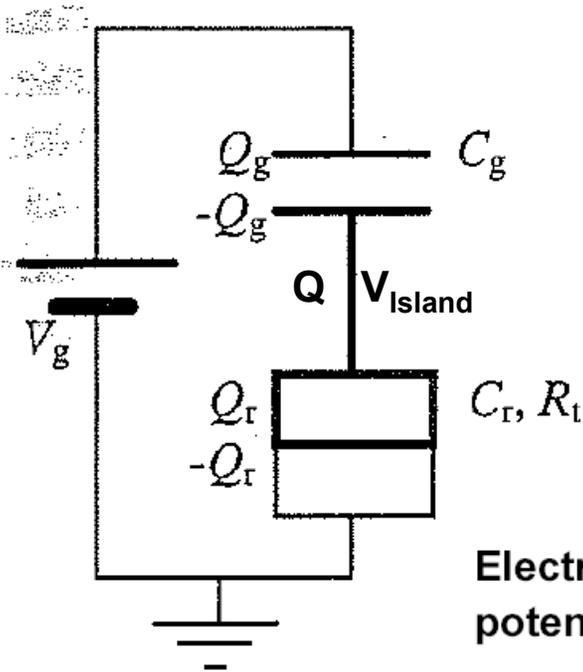
Electrostatics gives the following relation between the different potentials and the charge  $Q$  on the island ( $V_D = 0$ ):
