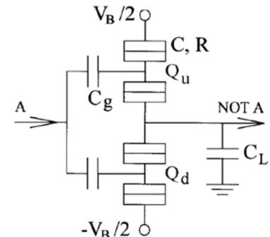
Figure 5. The complementary inverter made of two SET-transistors.
