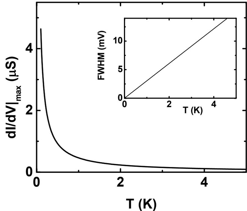
Left: Temperature dependence of the Coulomb peak height in the resonant transport model showing the characteristic increase as temperature is lowered. Right: peak height as a function of temperature. The inset shows the full width half maximum (FWHM) of the Coulomb peak as a function of temperature (see next slides). Calculations are performed with  $\Gamma = 10^9$  1/s and a gate coupling of 0.1 in the regime  $\Gamma < k_B T$ .
