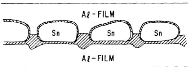
Sn disk –like metallic (superconducting) particles inbedded in aluminium-oxide matrix; diameter particles >2 nm
