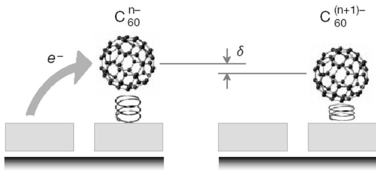
single electron tunneling events excite and probe the mechanical motion of the  $C_{60}$  bucky ball
