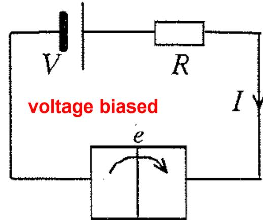
In practice, it is very difficult to establish current biasing in a single junction circuit. The impedance of air is of the order of hundred Ohms, thereby shunting the high resistance of the current source. One needs to create high resistances within a micron distance (otherwise shunting at high frequencies) of the junction to prevent this. One can use other tunnel junctions (SET transistor) or very thin disordered metals as leads.
